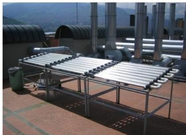
Fig. 1. Solar CPC system employed in this study. Source: GDCON Group Universidad de Antioquia.
