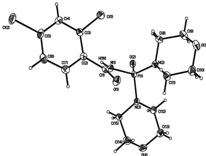
FIGURE 4 Molecular structure and atom-labeling scheme for compound **6a** (50% probability ellipsoids).
