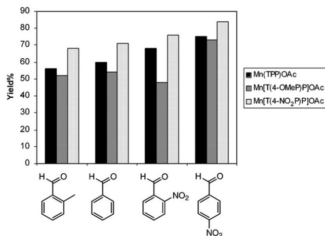
**Figure 1.** The comparison of catalytic activity of  $\text{Mn}(\text{TPP})\text{OAc}$ ,  $\text{Mn}[\text{T}(4\text{-OMeP})\text{P}]\text{OAc}$ , and  $\text{Mn}[\text{T}(4\text{-NO}_2\text{P})\text{P}]\text{OAc}$  in the oxidation of different benzyl alcohols with molar ratio of 100:100:10:1 for alcohol/oxidant/Py/catalyst in  $\text{CH}_2\text{Cl}_2$  after 5 min.
