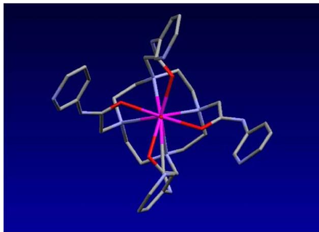
**Figure 2.** X-ray crystal structure of **2Eu** ( $\Delta(\lambda\lambda\lambda\lambda)$ ) showing the nine coordinate environment of the Eu(III) complex. Hydrogen atoms and triflate anions have been removed for clarity.
