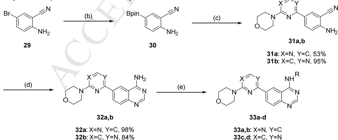
Reagents and conditions: (a) morpholine,  $K_2CO_3$ , THF, RT, 24 h; (b)  $B_2pin_2$ , KOAc, Pd(dppf)Cl<sub>2</sub>-DCM, 1,4-dioxane, MW, 130°C, 1 h, 88%; (c) **31a** or **31b**,  $Cs_2CO_3$ , Pd(PPh<sub>3</sub>)<sub>4</sub>, 1,4-dioxane/H<sub>2</sub>O (3:1), MW, 130°C, 10 min; (d) formamide, MW, 200°C, 1 h; (e) 2-chloropyrimidine or 4-chloropyridine, Pd<sub>2</sub>(dba)<sub>3</sub>, DPPF, 1,4-dioxane, MW, 170°C, 1-2 h, 30-67%.
