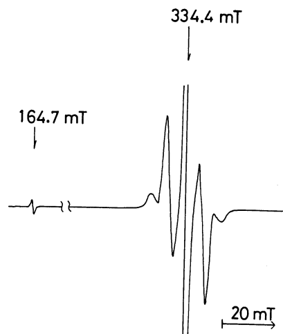
Fig. 6. Triplet ESR spectrum of 2d generated by photodissociation of its cyclomers in MTHF at -196^{\circ}\text{C} .
