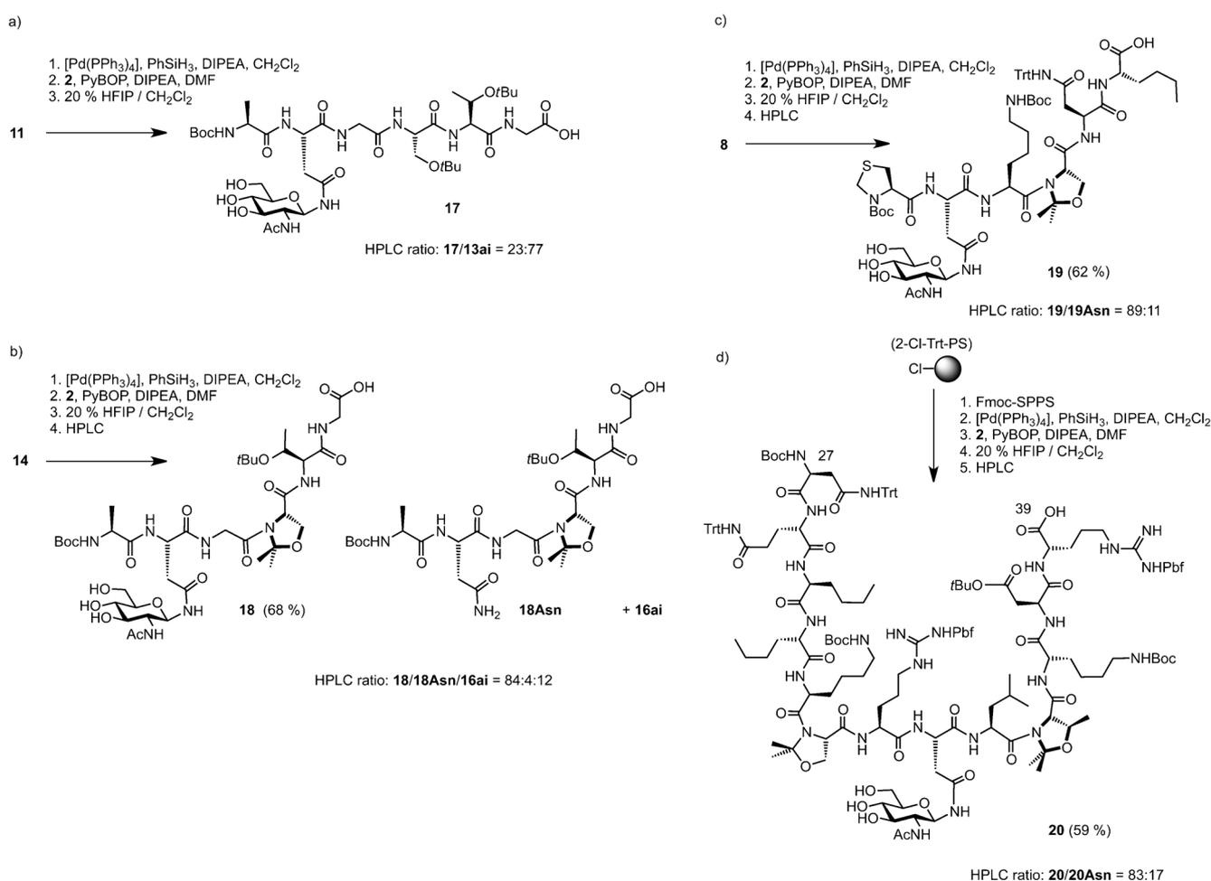
**Scheme 3.** Solid phase coupling of GlcNAc-NH<sub>2</sub> **2** to peptides. DIPEA = diisopropylethylamine, DMF = *N,N*-dimethylformamide, GlcNAc = *N*-acetylglucosamine, PyBOP = (benzotriazol-1-yloxy)tripyrrolidinophosphonium hexafluorophosphate.
