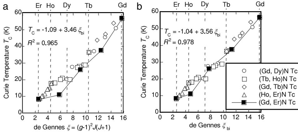
**Fig. 3.** Curie temperature of RE nitrides as a function of (a) the de Gennes factor  $\xi = (g - 1)^2 J(J + 1)$  and (b) the modified de Gennes factor  $\xi_{bi} = x^2 \xi_{Gd-Gd} + 2x(1 - x)\xi_{Gd-Er} + (1 - x)^2 \xi_{Er-Er}$ .
