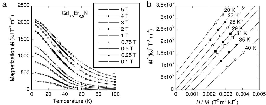
**Fig. 2.** (a) Magnetization data for  $Gd_{0.5}Er_{0.5}N$  under different magnetic fields. (b) Arrott plot of data obtained under fields of 5, 4, and 3 T at seven different temperatures.
