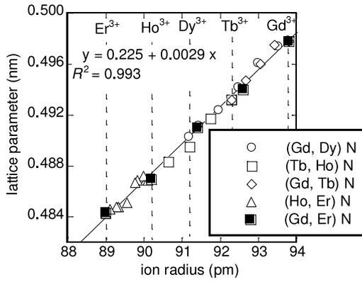
**Fig. 1.** Lattice parameter as a function of average radius for trivalent rare earth ions. The line was determined by the least mean square method.
