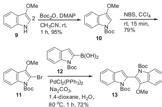
**Scheme 2.** Model study on the Suzuki coupling reaction.
