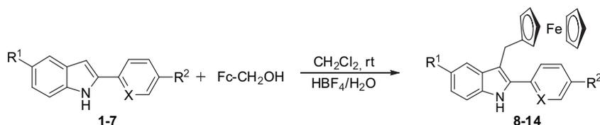
**Scheme 1.** Synthesis of ferrocene-indole hybrids **8–14**. Reagents and conditions: 2-arylidole (1 mmol), ferrocenemethanol (1 mmol), CH<sub>2</sub>Cl<sub>2</sub>, aqueous solution of HBF<sub>4</sub> (6 mL of 50% commercial acid + 4 mL of water), rt, 1 h.
