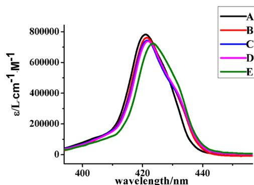
**Figure 2.** UV–vis spectra of [Zn<sub>2</sub>-III] in 0.1 mm, 1 mm, and 1.0 cm quartz cells at different concentrations in methylene chloride. The intensities are normalized on the basis of the concentrations of [Zn<sub>2</sub>-III]: (A) 1.5 × 10<sup>-7</sup> mol/L; (B) 6.0 × 10<sup>-7</sup> mol/L; (C) 1.5 × 10<sup>-6</sup> mol/L; (D) 1.5 × 10<sup>-5</sup> mol/L; (E) 1.5 × 10<sup>-4</sup> mol/L.
