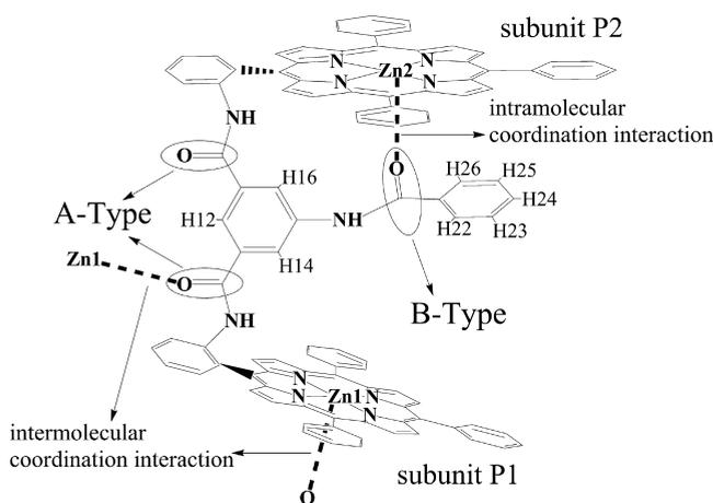
**Figure 5.** Proposed binding mode for  $[\text{Zn}_2\text{-III}]$ . The A-type carbonyl group involves “intermolecular” interactions, and the B-type carbonyl group involves “intramolecular” Zn–O coordination interactions.
