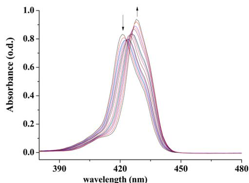
**Figure 3.** UV–vis spectral change of [Zn<sub>2</sub>-III] (1.50 × 10<sup>-6</sup> M) upon the addition of 1R as the host–guest molar ratios are from 1:0 to 1:850.
