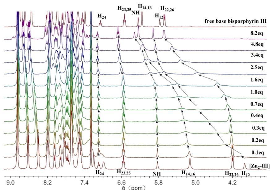
**Figure 6.**  $^1\text{H}$  NMR spectral changes of  $[\text{Zn}_2\text{-III}]$  ( $4.4 \times 10^{-3}$  M) upon the addition of **1R** in  $\text{CDCl}_3$  at 298 K as the host–guest molar ratios are from 1:0 to 1:8.2.
