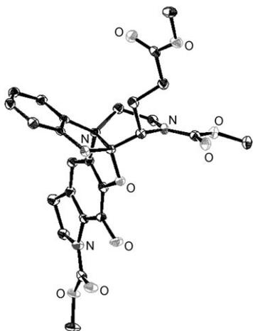
**Figure 2.** ORTEP drawing of **12**. Thermal ellipsoids are shown at the 50% probability level. One molecule of CH<sub>3</sub>CN per molecule of **12** observed in the crystal lattice is omitted for clarity.
