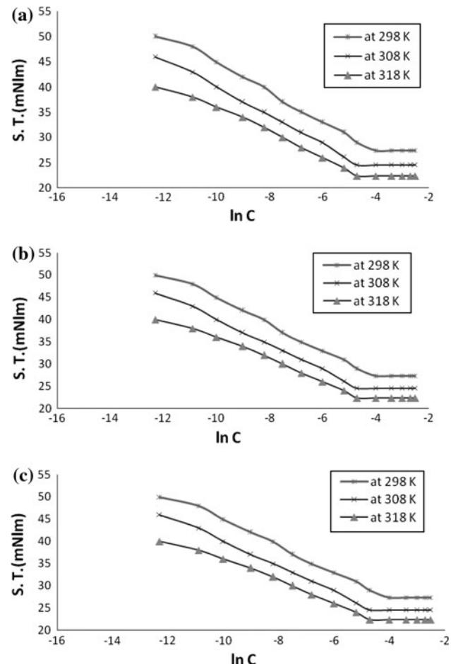
**Fig. 5** **a** S.T. conc. isotherm of SP6 at different temperatures, **b** S.T. conc. isotherm of SP8 at different temperatures, **c** S.T. conc. isotherm of SP10 at different temperatures
