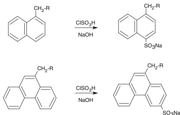
**Fig. 2 a, b** The sulfonation reactions of alkynaphthalene and alkylphenanthrene
