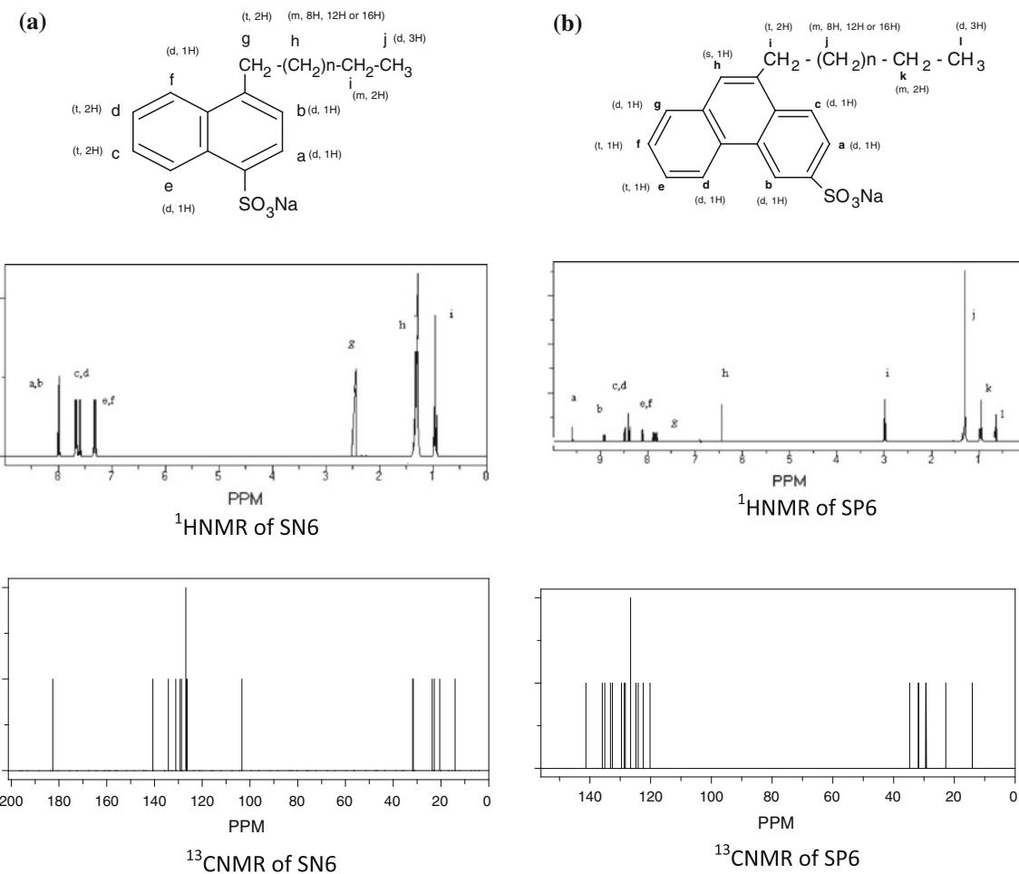
**Fig. 3** a and b <sup>1</sup>H NMR and <sup>13</sup>C NMR for SN6 and SP6
