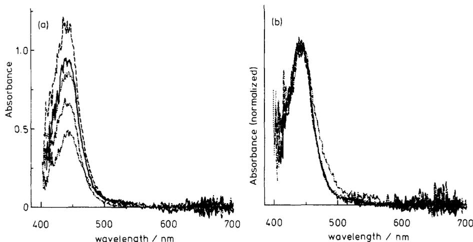
**Figure 3.** Transient absorption spectra recorded at 5 ns after excitation for the all-trans (—), 7-cis (···), 9-cis (---), 11-cis (- - -), and 13-cis (- · - ·) isomers. Spectra (a) before and (b) after normalization at  $\lambda_{\text{max}}$ .
