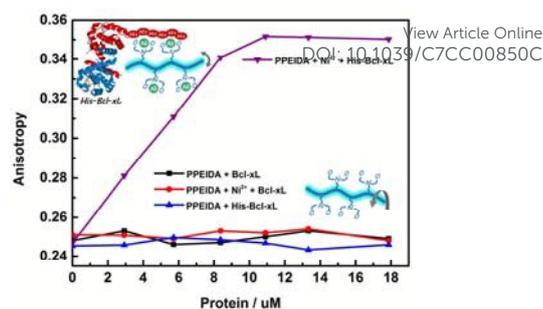
**Fig. 2** Fluorescence anisotropy of PPEIDA in response to varying concentrations of Bcl-xL or His-tagged Bcl-xL in the presence or absence of  $\text{Ni}^{2+}$ ; schematic diagram of fluorescence anisotropy variation.
