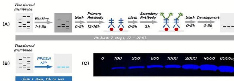
**Fig. 4** Procedure comparison of (B) our method to the (A) conventional Western blot analysis. (C) Results of PPEIDA-Ni<sup>2+</sup> complex-based Western blot analysis for His-tagged protein detection. Protein quantities over a range from 100 to 6000 ng.
