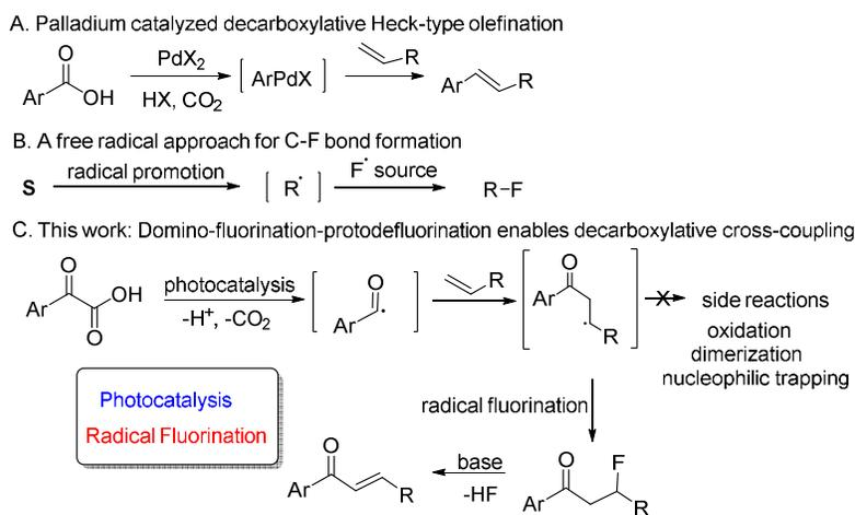
**Scheme 1.** A) Palladium catalyzed decarboxylative Heck-type olefination. B) Free radical methods for fluorine incorporation. C) Our strategy for photoredox catalysis decarboxylative cross-coupling combined with radical fluorination.
