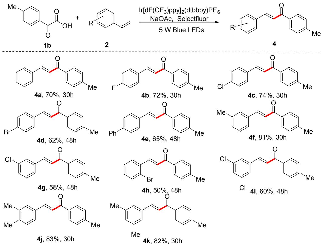
Reaction conditions: **1b** (0.2 mmol), **2** (0.4 mmol, 2.0 equiv), Ir[dF(CF<sub>3</sub>)ppy]<sub>2</sub>(dtbbpy)PF<sub>6</sub> (0.002 mmol, 2 mol %), NaOAc (0.4 mmol, 2.0 equiv), CH<sub>3</sub>CN/H<sub>2</sub>O (V/V = 1:1, 2 mL), Selectfluor (0.5 mmol, 2.5 equiv), at room temperature, 5 W blue LEDs, 30 - 48 h.
