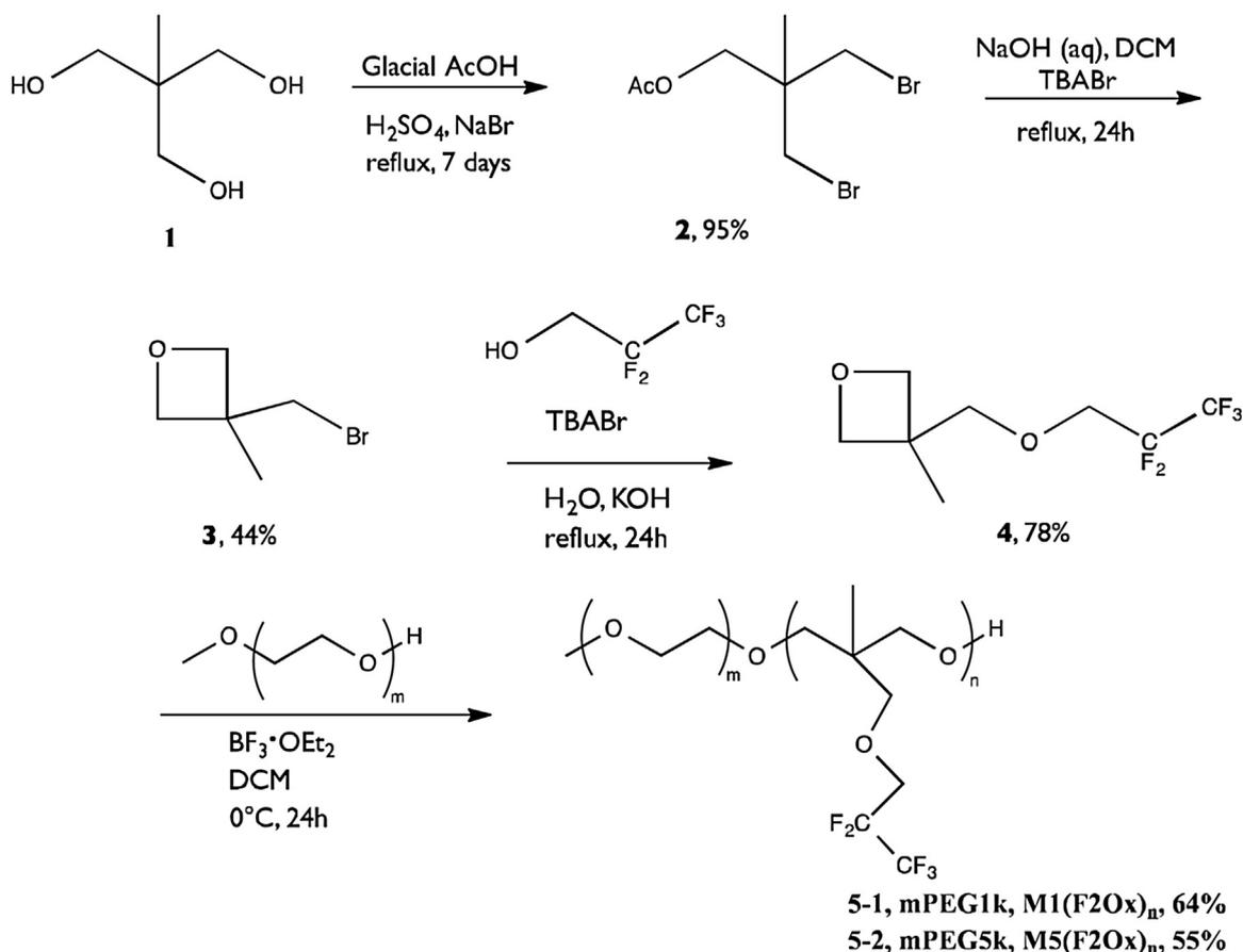
Scheme 1. Synthesis of  $M_x(F_2Ox)_y$ . Note on nomenclature: M corresponds to mPEG, with the following number being the average molecular weight. (F2Ox) indicates the opened oxetane monomer with a perfluoroethyl side chain.
