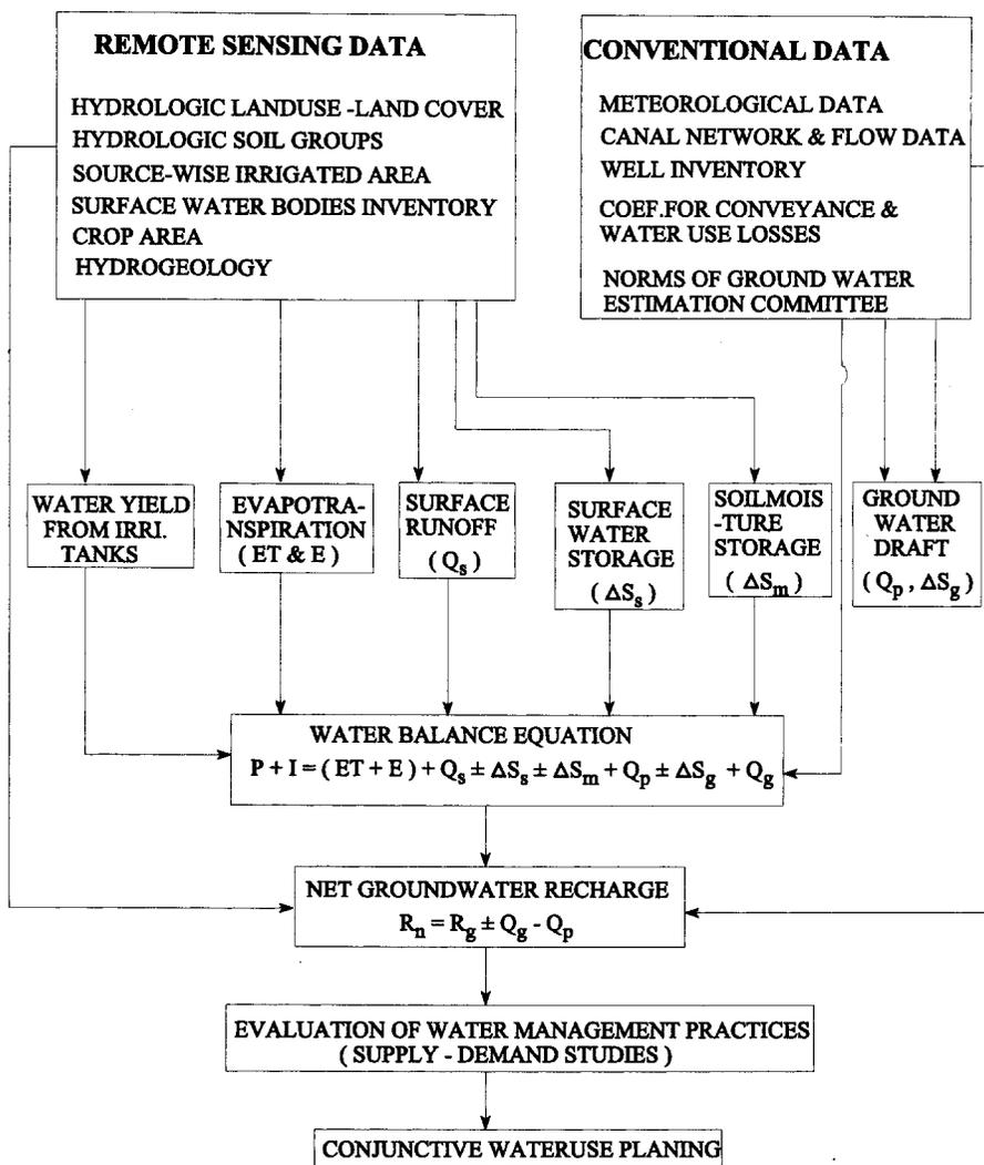
Figure 4. Methodology to estimate net groundwater recharge from the water balance study using satellite data and ancillary data for conjunctive water use planning.
