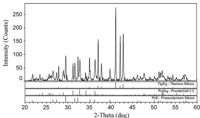
**Fig. 5.** XRD pattern of the equilibrated alloy (14 at.% Pr, 46 at.% Ti and 40 at.% Si) indicating the existence of  $Ti_5Si_3$ , PrSi and  $Pr_5Si_4$ .
