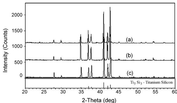
**Fig. 6.** The XRD patterns of some equilibrated Pr–Ti–Si ternary system samples: (a) 62 at.% Ti and 38 at.% Si; (b) 62.5 at.% Ti and 37.5 at.% Si; and (c) 63 at.% Ti and 37 at.% Si.
