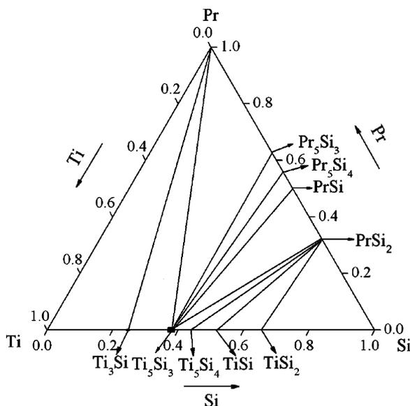
**Fig. 7.** The isothermal section of phase diagram of Pr–Ti–Si ternary system at 773 K.
