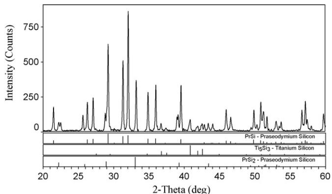
**Fig. 2.** XRD pattern of the equilibrated alloy (36 at.% Pr, 14 at.% Ti and 50 at.% Si) indicating the existence of Ti<sub>5</sub>Si<sub>3</sub>, PrSi<sub>2</sub> and PrSi.
