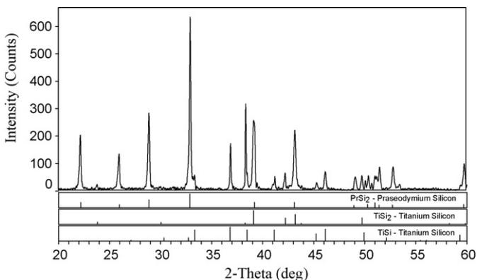
**Fig. 4.** XRD pattern of the equilibrated alloy (12 at.% Pr, 28 at.% Ti and 60 at.% Si) indicating the existence of TiSi<sub>2</sub>, TiSi and PrSi<sub>2</sub>.
