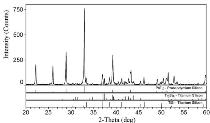
**Fig. 3.** XRD pattern of the equilibrated alloy (14 at.% Pr, 30 at.% Ti and 56 at.% Si) indicating the existence of Ti<sub>5</sub>Si<sub>4</sub>, TiSi and PrSi<sub>2</sub>.
