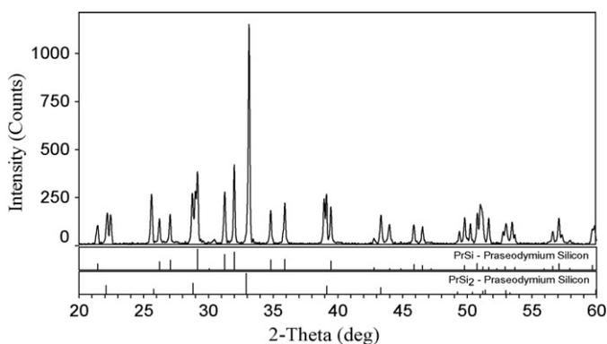
**Fig. 1.** XRD pattern of the equilibrated alloy (42.86 at.% Pr and 57.14 at.% Si) indicating the existence of PrSi<sub>2</sub> and PrSi.
