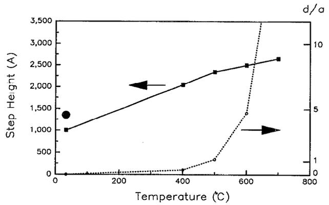
FIG. 3. Step heights of ion etched surfaces of TiSi<sub>2</sub> after 15 min ion beam etching, as a function of temperature from 33 to 700 °C. The height determined from RBS measurement at 33 °C is shown as an added data point. The dotted curve shows the ratio of diffusion length to sputtered thickness in 1 s for Si diffusing through TiSi<sub>2</sub>.
