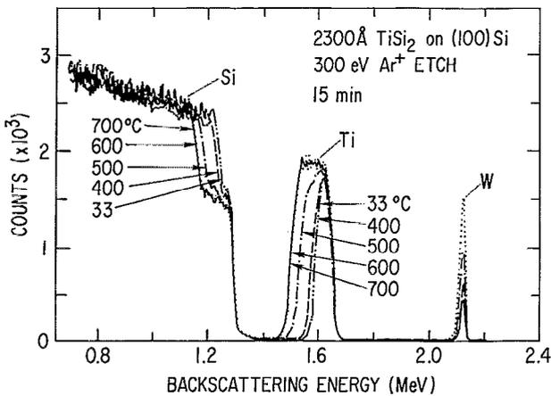
FIG. 2. Rutherford backscattering spectra of TiSi<sub>2</sub> films on Si (shown in Fig. 1) after 15 min Ar<sup>+</sup> ion beam etching at temperatures of 33–700 °C. The spectra of nonetched samples and those etched at 600 and 700 °C are indistinguishable.
