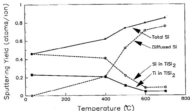
FIG. 5. Absolute sputtering yields of Ti and Si vs temperature for 300 eV  $\text{Ar}^+$  ion bombardment of 2300-Å thick  $\text{TiSi}_2$  layer on Si. The Ti yield is from Ti sputtered from  $\text{TiSi}_2$ . The Si yield shown as the component sputtered from  $\text{TiSi}_2$ , the component supplied by diffusion, and the total Si yield.
