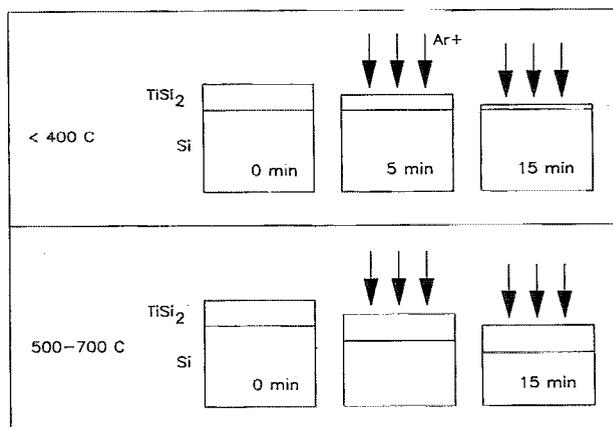
FIG. 6. Schematic diagram indicating sputtering of  $\text{TiSi}_2$  layer on Si at low temperature (<400 °C) and at high temperature (500–700 °C). At high temperature, the  $\text{TiSi}_2$  layer thickness remains almost unchanged.
