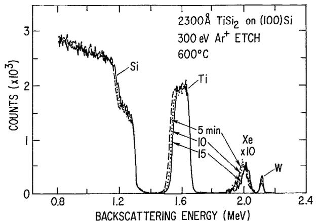
FIG. 4. Rutherford backscattering spectra of Xe-implanted TiSi<sub>2</sub> on Si after ion beam etching for 5, 10, and 15 min at 600 °C. The region showing the Xe marker is magnified by 10.
