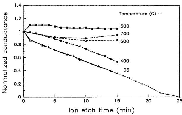
FIG. 1. Normalized sheet conductance vs time for 2300 Å thick TiSi<sub>2</sub> on Si, during Ar<sup>+</sup> ion beam etching (300 eV, 0.27 mA/cm<sup>2</sup>) at temperatures of 33–700 °C.
