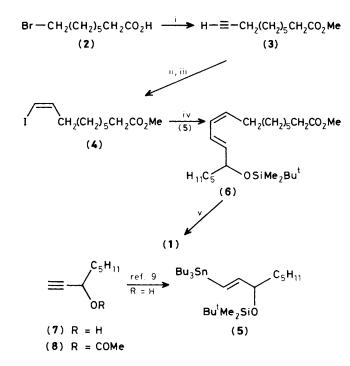
Scheme 1. Reagents: i, LiC=CH/(CH<sub>2</sub>NH<sub>2</sub>)<sub>2</sub>, NH<sub>3</sub>, -33 °C, 10 h, then MeOH, H<sup>+</sup>; ii, NaOMe then I<sub>2</sub>; iii, [=NCO<sub>2</sub>K]<sub>2</sub>, HOAc in MeOH, Bu<sup>n</sup>NH<sub>2</sub> then chromatography [33.5% from (2)]; iv, Pd(PPh<sub>3</sub>)<sub>2</sub>Cl<sub>2</sub>, HCONMe<sub>2</sub>, 60 °C under N<sub>2</sub>, 4 days (60%); v, TBAF, then K<sub>2</sub>CO<sub>3</sub>, H<sub>2</sub>O, MeOH.
