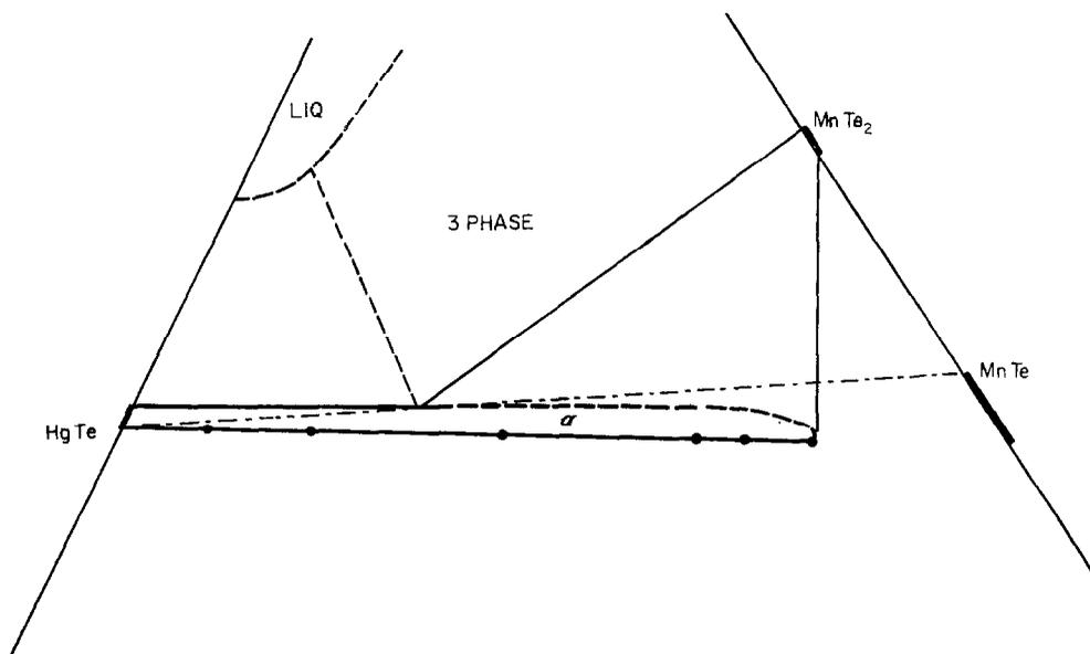
FIG. 4. Ternary isotherm at  $550^\circ\text{C}$  showing the  $\alpha$ -phase region. ——— Construction line joining stoichiometric compositions HgTe and MnTe.
