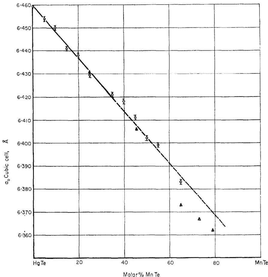
FIG. 3. Variation in structure cell dimensions of  $\alpha$ -phases with change in composition.
