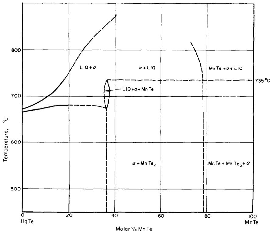
FIG. 2. HgTe-MnTe section of the ternary phase diagram.
