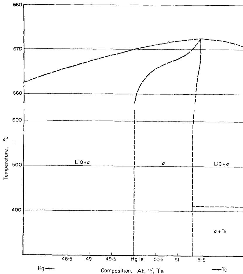
FIG. 1. Schematic phase diagram for the system Hg-Te, at the composition HgTe.
