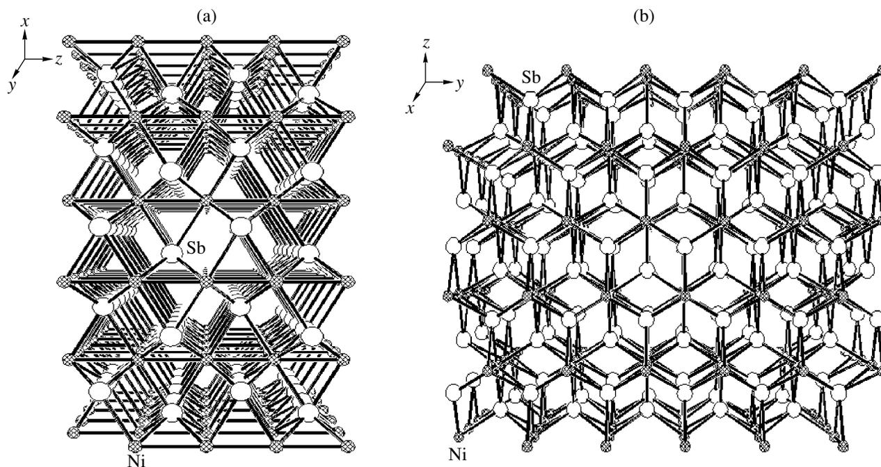
Fig. 3. Crystal structure of NiSb projected along the (a) [010] and (b) [100] directions.
