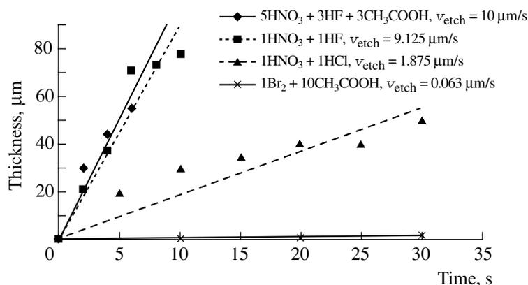
Fig. 4. Thickness of the layer removed from the NiSb surface as a function of etching time for different etchants.
