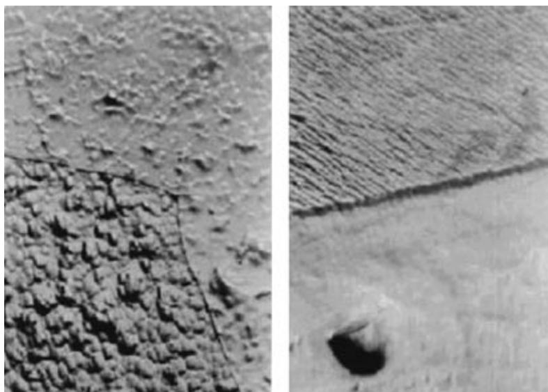
Fig. 5. NiSb surfaces etched with a 1 : 1 mixture of HNO<sub>3</sub> and HF; 200 $\times$ .
