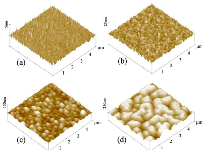
FIG. 1.  $5 \times 5\ \mu\text{m}^2$  AFM images of InN samples grown at  $350\ ^\circ\text{C}$  (a),  $400\ ^\circ\text{C}$  (b),  $450\ ^\circ\text{C}$  (c), and  $500\ ^\circ\text{C}$  (d), respectively.
