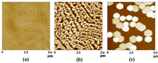
FIG. 4.  $5 \times 5 \mu\text{m}^2$  AFM images of the surfaces of the as-grown GaN layer (a) and the thin InN films with a nominal thickness of about 40 nm grown at 400 °C (b), and 500 °C (c), respectively.
