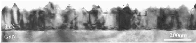
FIG. 2. Cross-sectional bright-field TEM image of InN film observed along the  $[11\bar{2}0]$  direction with  $g=(10\bar{1}0)$ .
