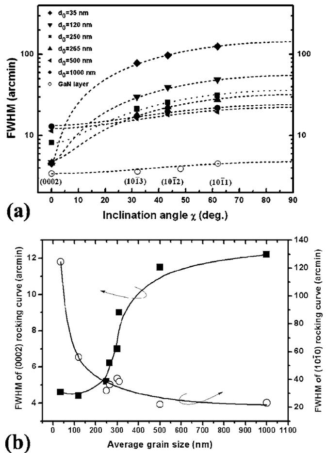
FIG. 3. (a) FWHM of x-ray rocking curves measured in a skew symmetric geometry as a function of the lattice plane inclination angle with respect to (0002). The dashed lines are fitting curves. (b) FWHM of (0002) rocking curves (filled squares) and the extrapolated FWHM of (10 $\bar{1}$ ) rocking curves (filled circles) as a function of average grain size.
