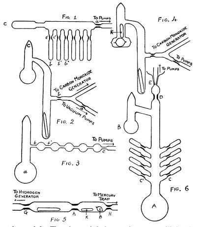
ately resealed. The tube was baked out under vacuum, filled with carbon monoxide, and again evacuated. The pumps were sealed off at the capillary a, and the tube was filled with carbon monoxide to 60 cm. pressure. It was sealed off at b, and heated at 400°, the phosphorus pentoxide compartment being meanwhile cooled. In order to examine a tube, the bulb of oxide was broken by allowing it to fall on to the bottom of the tube, the pentoxide compartment
