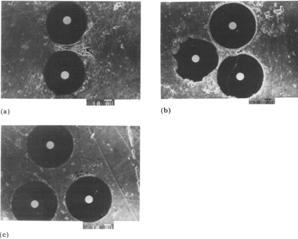
Fig. 4. Scanning electron micrographs of Al-60vol.%B composite: aluminium temperature, 700 °C; treatment time, 5 min. (a) Initial fibre. TiB<sub>2</sub> fibre coated (deposit thickness, 0.4 μm) by (b) BCl<sub>3</sub>-TiCl<sub>4</sub>-H<sub>2</sub> CVD process (800 °C, 20 s) and (c) B-TiCl<sub>4</sub>-H<sub>2</sub> CVD process (800 °C, 2 min).
