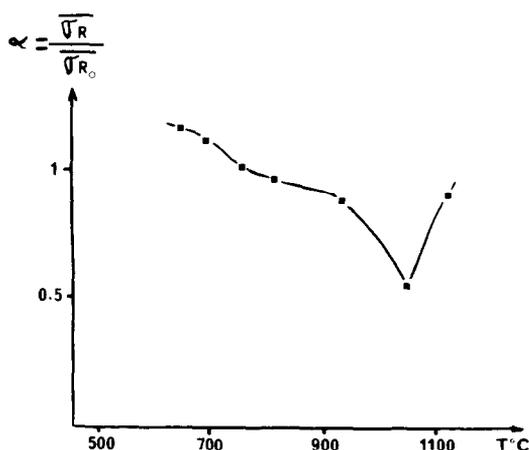
Fig. 3. Relation between relative tensile strength and temperature of the substrate.
