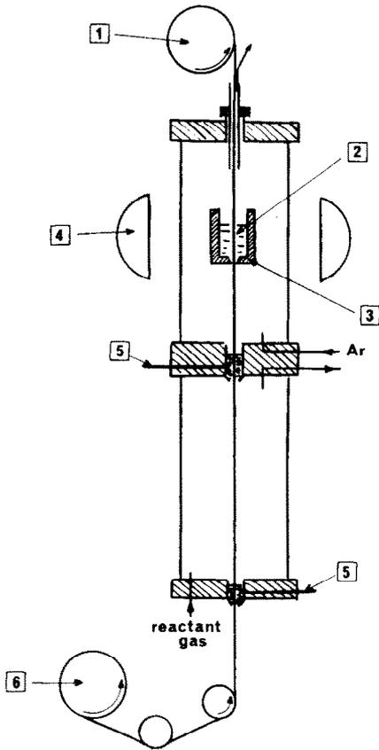
Fig. 2. Schematic diagram of the deposition reactor: 1, drive pulley; 2, molten aluminium; 3, graphite crucible; 4, image furnace with elliptical mirrors and halogen lamps; 5, current leads; 6, spooling and tension pulleys.
