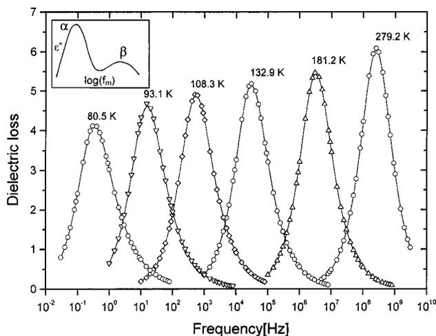
FIG. 1. Typical dielectric loss spectra of  $\text{TiNO}_2$  showing a single relaxation peak at all temperatures. The inset is an illustration of the generally observed bimodal relaxation in viscous liquids and glasses, and in supercooled plastic crystals.
