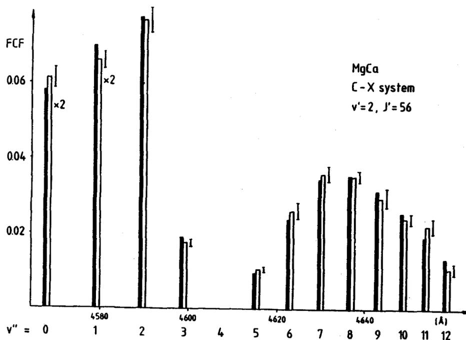
FIG. 4. Comparison of the measured (open bars) and calculated (solid bars) Franck-Condon factors for two  $v''$  progressions of the C-X system.
