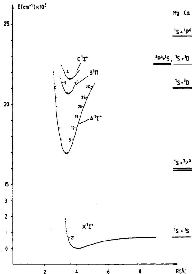
FIG. 7. Potential energy curves of the  $X$ ,  $A$ ,  $B$ , and  $C$  states of the MgCa molecule.
