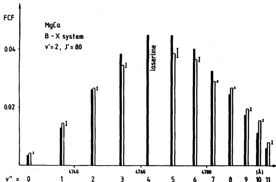
FIG. 6. Comparison of the measured (open bars) and calculated (solid bars) Franck-Condon factors for two  $v''$  progressions of the B-X system.
