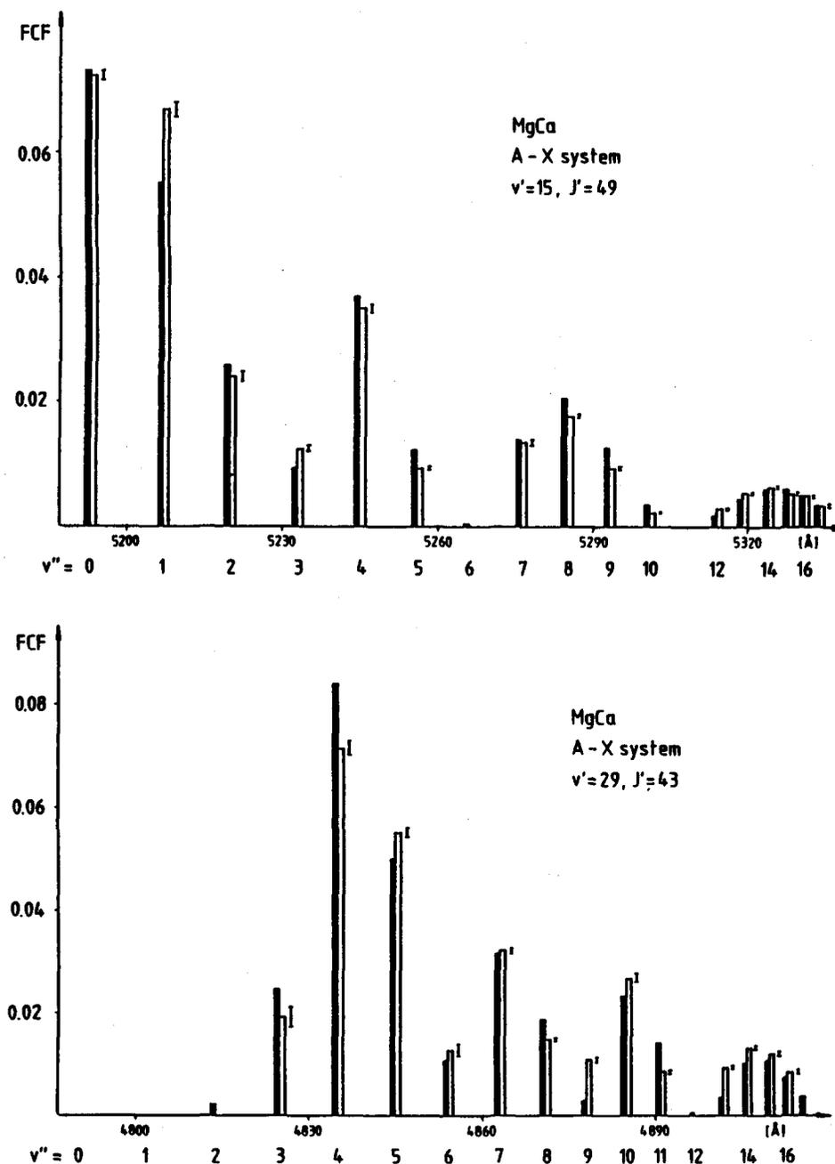
FIG. 5. Comparison of the measured (open bars) and calculated (solid bars) Franck-Condon factors for two  $v''$  progressions of the A-X system. As explained in the text, the calculated Franck-Condon factors originate from an RKR potential, which is based on a preliminary set of Dunham-type coefficients, which differ from the ones given in Table V and which have been determined in a least squares fit including the perturbed levels with  $28 < v' < 33$ .
