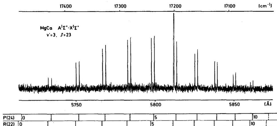
FIG. 2. Laser induced fluorescence spectrum excited by a stabilized single mode dye laser at 581.18 nm.
