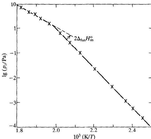
FIGURE 5. Second-law determination of the melting enthalpy  $\Delta_{\text{fus}}H_m^\circ$  from measurements on  $2\text{InCl}_2(\text{s or l}) = \text{In}_2\text{Cl}_4(\text{g})$ .
