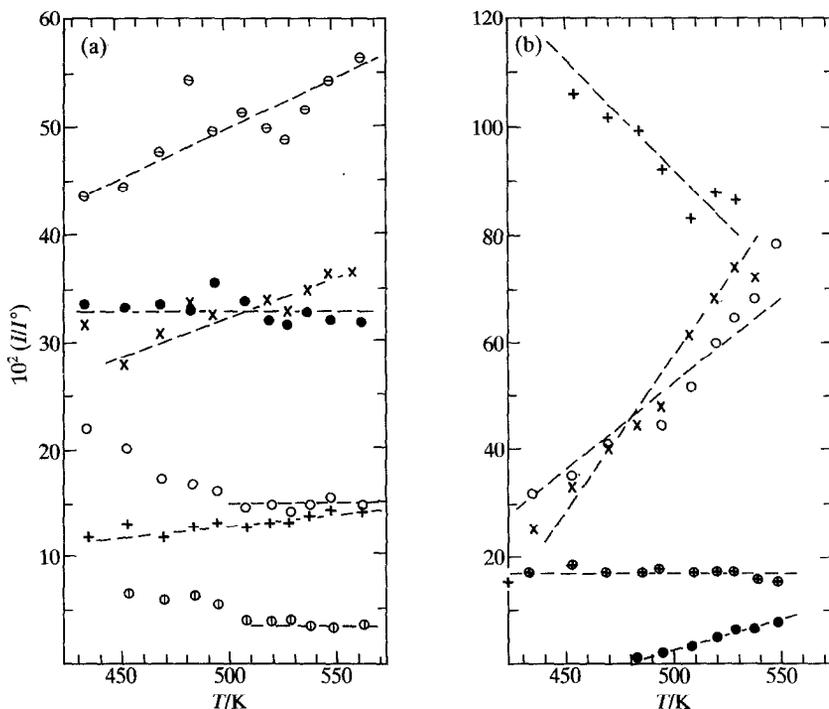
FIGURE 1. Ion-intensity ratios measured at 60 V from the vapour phase in equilibrium with  $\text{InCl}_2(\text{s or l})$  as a function of temperature.
