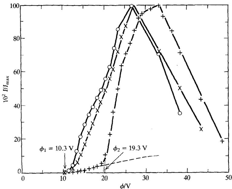
FIGURE 2. Normalized ionization-efficiency curves for  $\text{In}_2\text{Cl}_4^+$  as measured from vapours in equilibrium with different condensed phases:  $\circ$ ,  $\text{InCl}(s)$ ;  $\times$ ,  $\text{InCl}_2(s)$ ; and  $+$ ,  $\text{InCl}_3(s)$ .  $\phi_1$  is the ionization potential of  $\text{In}_2\text{Cl}_4(g)$ , while  $\phi_2$  is the fragmentation threshold observed for the appearance of  $\text{In}_2\text{Cl}_4^+$  from  $\text{In}_2\text{Cl}_6(g)$ .
