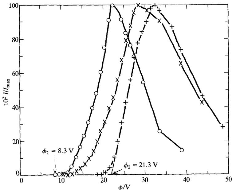
FIGURE 3. Normalized ionization-efficiency curves for  $\text{InCl}^+$  as measured from vapours in equilibrium with different condensed phases:  $\circ$ ,  $\text{InCl}(\text{s})$ ;  $\times$ ,  $\text{InCl}_2(\text{s})$ ; and  $+$ ,  $\text{InCl}_3(\text{s})$ .  $\phi_1$  is the ionization potential of  $\text{InCl}(\text{g})$  while  $\phi_2$  is the fragmentation threshold observed for the appearance of the fragment  $\text{InCl}^+$  from  $\text{InCl}_3(\text{g})$ .
