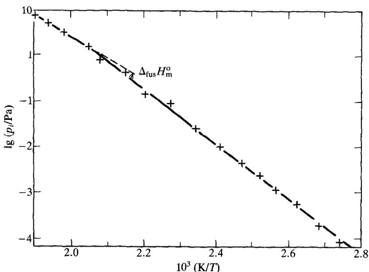
FIGURE 4. Second-law determination of the melting enthalpy  $\Delta_{\text{fus}}H_m^\circ$  from measurements on  $\text{InCl}(\text{s or l}) = \text{InCl}(\text{g})$ .
