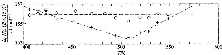
FIGURE 6. Influence of the choice of the melting enthalpy  $\Delta_{\text{fus}}H_m^\circ$  on the deduced third-law standard enthalpies for the reaction:  $2\text{InCl}_2(\text{s}) = \text{In}_2\text{Cl}_4(\text{g})$ : +, with  $\Delta_{\text{fus}}H_m^\circ = 20.92 \text{ J} \cdot \text{mol}^{-1}$  estimated from reference 31; O, with  $\Delta_{\text{fus}}H_m^\circ = 34.94 \text{ J} \cdot \text{mol}^{-1}$ , the mean value of our second-law results from reaction (6).
