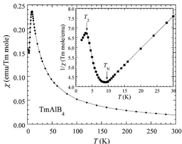
Fig. 1. Temperature dependence of the magnetic susceptibility  $\chi$  of  $\beta$ -type  $\text{TmAlB}_4$ . The inset is an enlarged view of the inverse susceptibility at low temperatures.
