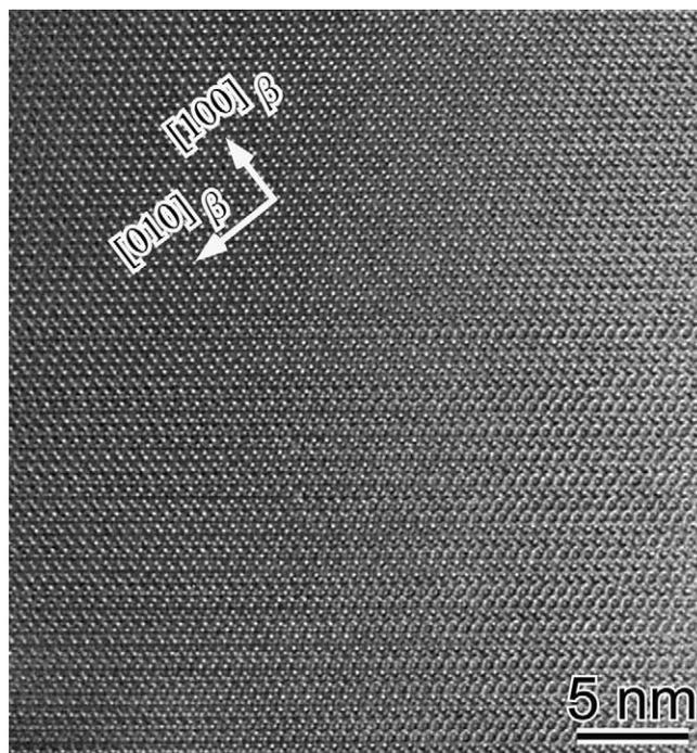
Fig. 3. A many-beam bright-field TEM image taken with the incident electron beam parallel to the  $[001]$  direction.
