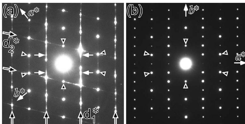
Fig. 2. ED patterns of (a)  $\beta$ - and (b)  $\alpha$ -type phases taken with the incident electron beam parallel to the  $[001]$  direction. White arrows in (a) indicate reflection positions of the  $\alpha$ -type phases. Large arrows in (a) indicate characteristic diffuse streaks. The  $\alpha$ - and  $\beta$ -type phases belong to orthorhombic systems, space groups  $Pbam$  and  $Cmmm$ , respectively.
