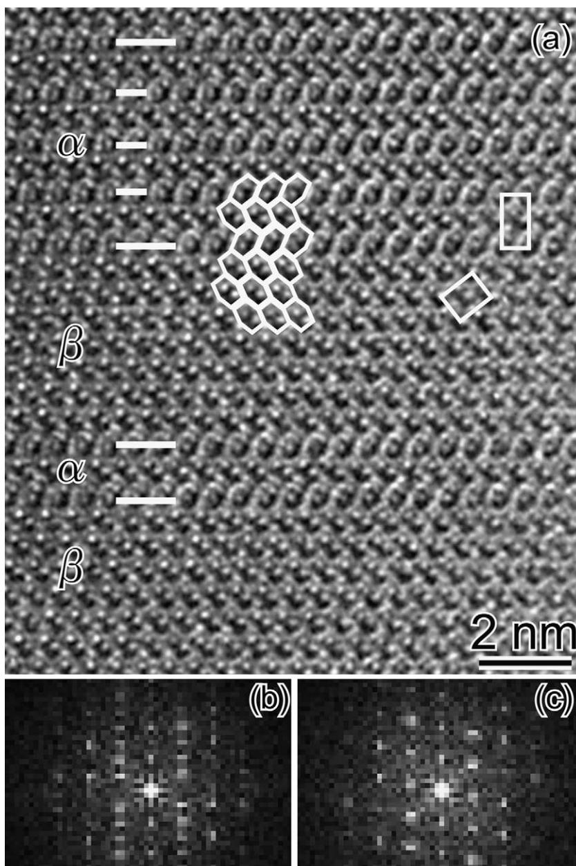
**Fig. 4.** An enlarged HREM image from a part of the intergrowth nanostructure. Deformed hexagons in (a) correspond to the structural unit in Fig. 5(a). The upper and lower rectangles in (a) indicate unit cells of the  $\alpha$ - and  $\beta$ -type structures, respectively. Power spectra in (b) and (c) were obtained from regions of  $\alpha$ - and  $\beta$ -type phases, respectively.
