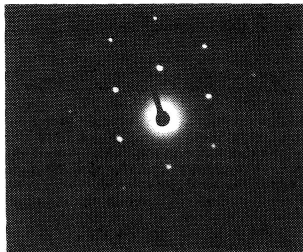
FIG. 4. Transmission electron diffraction pattern of the laser deposited GaP. The zone axis is  $\{110\}$ .
