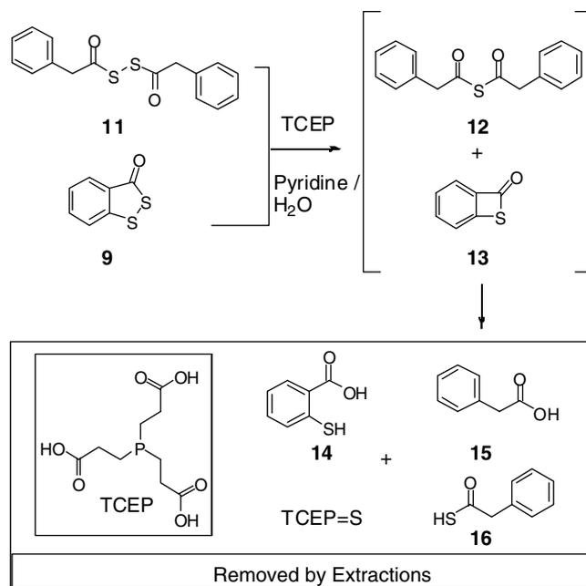
Scheme 2. Quenching of excess sulfur transfer reagents (putative products).<sup>17,20</sup>
