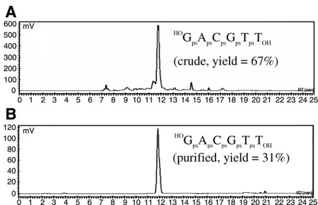
Fig. 2. HPLC trace (254 nm) of: (A) crude PS-hexamer **17**, (B) purified **17**.
