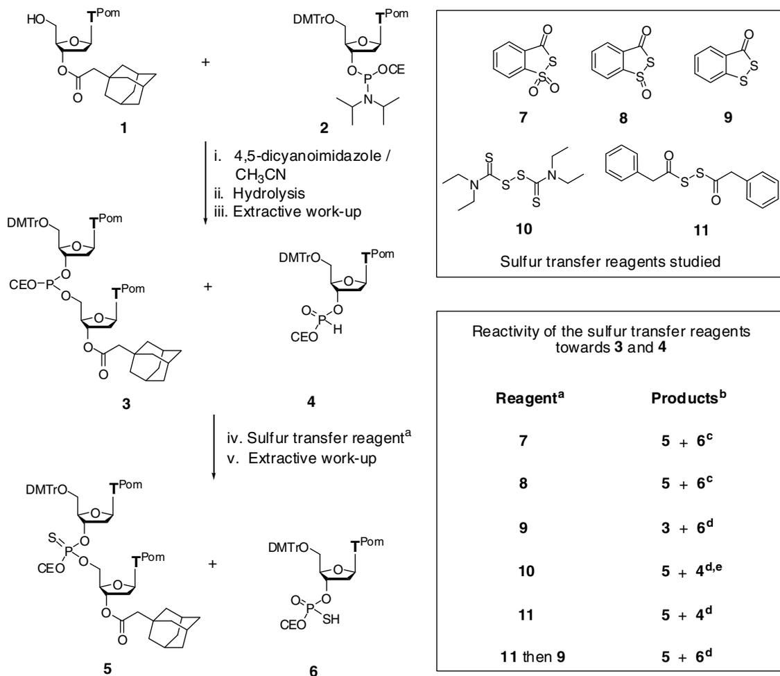
Scheme 1. Sulfurization strategy for phosphorothioates synthesis compatible with extractive purification. (a) Evaluated sulfur transfer reagents; (b) judged by <sup>31</sup>P NMR analysis; (c) 2.25 equiv sulfur transfer reagent, 2% H<sub>2</sub>O/pyridine, 30 min, approximately 11% of oxidized by-product<sup>26</sup> was detected; (d) 1.5 equiv sulfur transfer reagent, dry CH<sub>3</sub>CN, 30 min; (e) approximately 2% of oxidized by-product<sup>26</sup> was detected.
