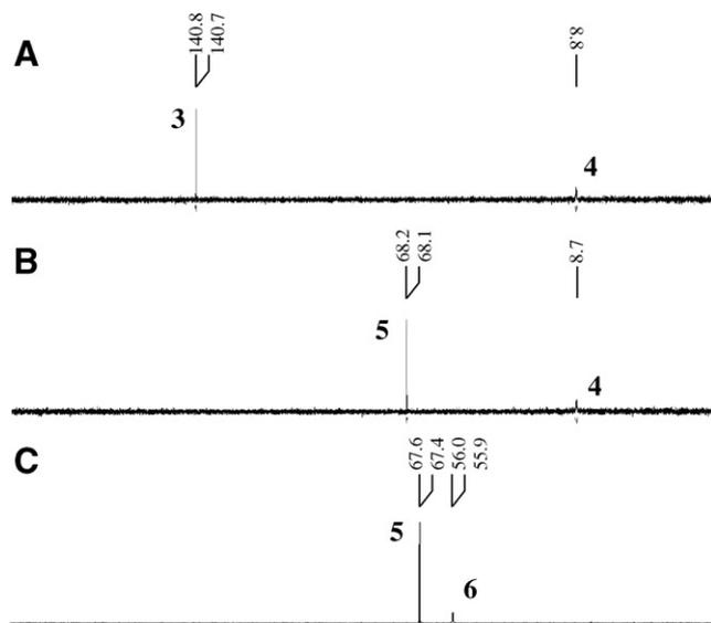
Fig. 1.  $^{31}\text{P}$  NMR spectra of the two-step sulfurization.  $^{31}\text{P}$  NMR (80.7 MHz,  $\text{CH}_3\text{CN}$  and  $\text{H}_3\text{PO}_4$  as internal standard) spectra of (A) the reaction mixture after dicyanoimidazole mediated coupling and subsequent hydrolysis of the excess phosphoramidite monomer **2**, (B) the reaction mixture after the addition of PADS (**11**), (C) the reaction mixture after the sequential addition of PADS (**11**) and reagent **9**.
