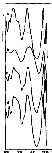
Fig. 2. IR spectra of a. starting hexavanadates, final pro- duct of heating b. K-, c. Rb-, d. Cs-salt
