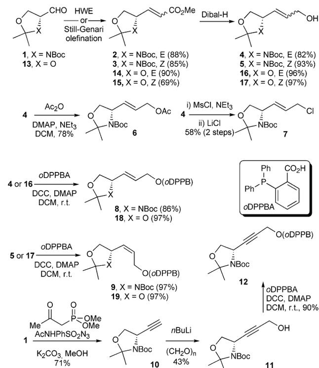
Scheme 1. Preparation of substrates for the copper-mediated allylic substitution reaction.
