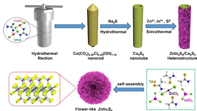
**Scheme 1.** Schematic illustration of the fabrication process of hierarchical  $\text{Co}_9\text{S}_8/\text{ZnIn}_2\text{S}_4$  tubular photocatalyst.
