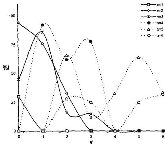
Fig. 3. Plot of oxoacetate cluster intensities against oxygen content,  $y$ , for  $[Gd_2O_3(CH_3COO)_x(H_2O)_y]_2 \cdot 3H_2O$ : — experiment done under dry conditions; ..... experiment done under wet matrix conditions.
