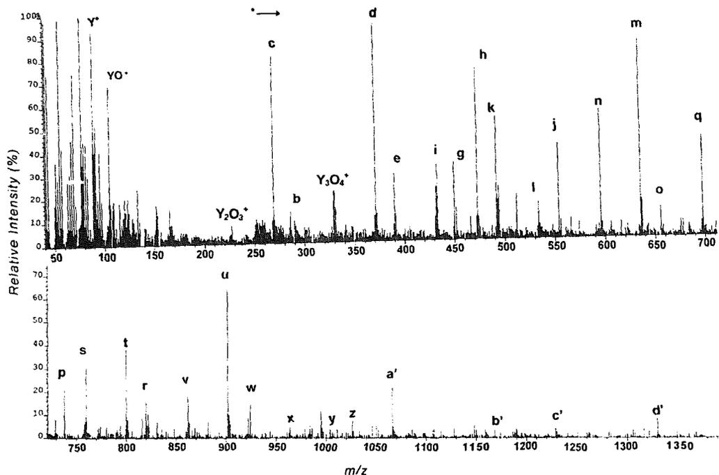
Fig. 2. The FAB MS spectrum of  $[Y(CH_3COO)_x(H_2O)_y]_2 \cdot 3H_2O$  in a *m*-NBA matrix; sensitivities after  $\ast \rightarrow \cdot \times 3$ .
