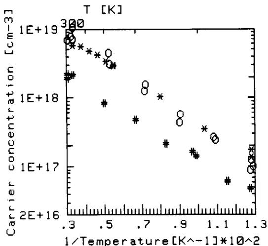
Fig. 2. Carrier concentration of  $TiS_3$  samples above 80 K samples plotted vs.  $100/T$  on an expanded scale.
