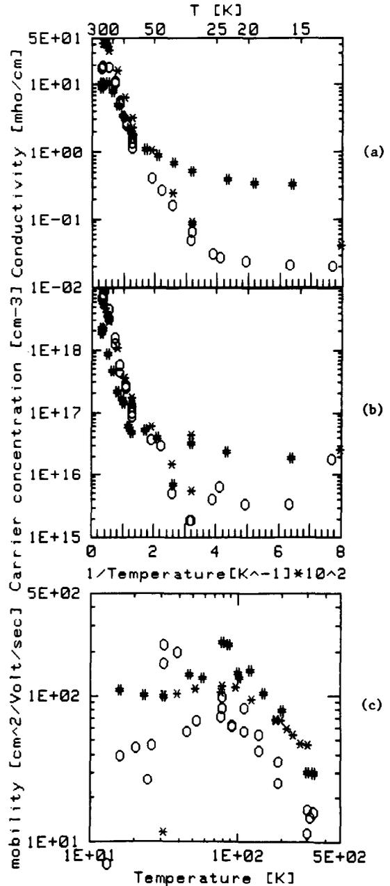
Fig. 1. Conductivity (a) and carrier concentration (b) plotted vs. 100/T and Hall mobility (c) plotted vs. T for  $TiS_3$  samples. Various symbols represent different samples.
