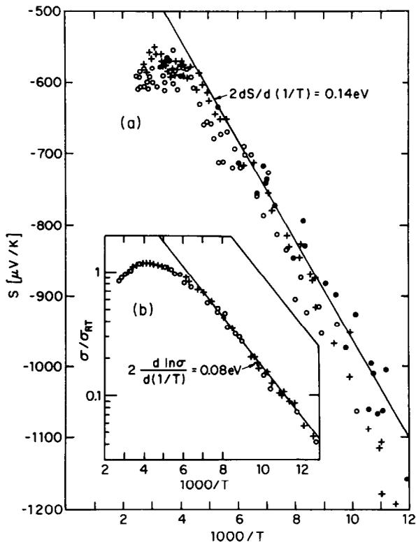
Fig. 3. Seebeck coefficient of  $TiS_3$  samples plotted vs.  $1000/T$  (a). Two lead resistance plotted vs.  $1000/T$  (b) for the same samples.
