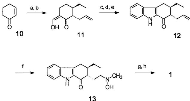
Scheme 4. a) 1. EtMgBr, CuI, Me<sub>2</sub>S, THF; 2. H<sub>2</sub>C=CHCH<sub>2</sub>Br, hexamethylphosphoric acid triamide (HMPT) (60%); b) NaH, glyme, HCOOEt (95%); c) PhN<sub>2</sub>Cl (85%); d) HCOOH (86%); e) NaOMe, MeOH, RT, 12–14 d (99%); f) 1. OsO<sub>4</sub>, NaIO<sub>4</sub>, MTBE, H<sub>2</sub>O; 2. MeNHOH, NaCNBH<sub>3</sub>, *i*PrOH, pH = 6 (85%); g) MeLi, THF, –20 °C → RT (98%); h) Ac<sub>2</sub>O, pyridine, 3 h, RT (99%).
