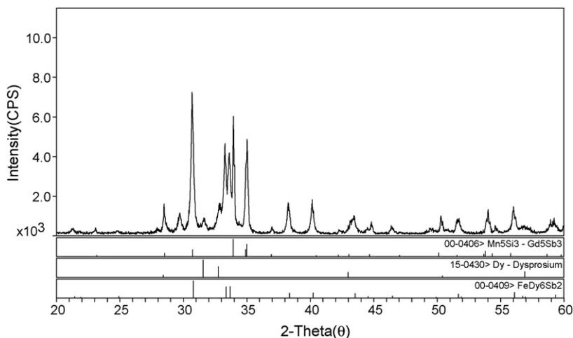
Fig. 3. XRD of sample with composition  $\text{Fe}_6\text{Dy}_{74}\text{Sb}_{20}$ :  $\text{Dy}_5\text{Sb}_3 + \text{Dy} + \text{FeDy}_6\text{Sb}_2$ .
