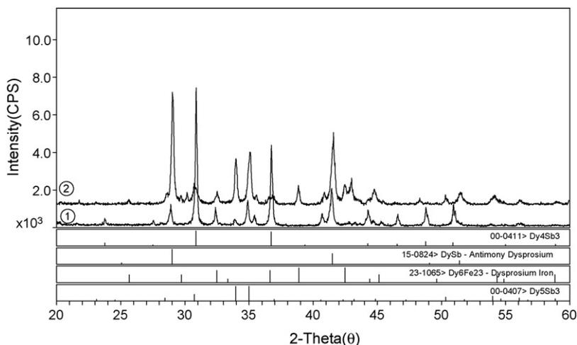
Fig. 1. XRD of sample with composition  $\text{Fe}_{54}\text{Dy}_{31}\text{Sb}_{15}$  under different annealed times: (1) XRD of the samples which were only annealed at 773 K for 10 days:  $\text{Dy}_4\text{Sb}_3 + \text{Dy}_5\text{Sb}_3 + \text{DySb} + \text{Fe}_{23}\text{Dy}_6$ ; (2) XRD of the samples after annealing at 773 K for 10 days again:  $\text{Dy}_5\text{Sb}_3 + \text{DySb} + \text{Fe}_{23}\text{Dy}_6$ .
