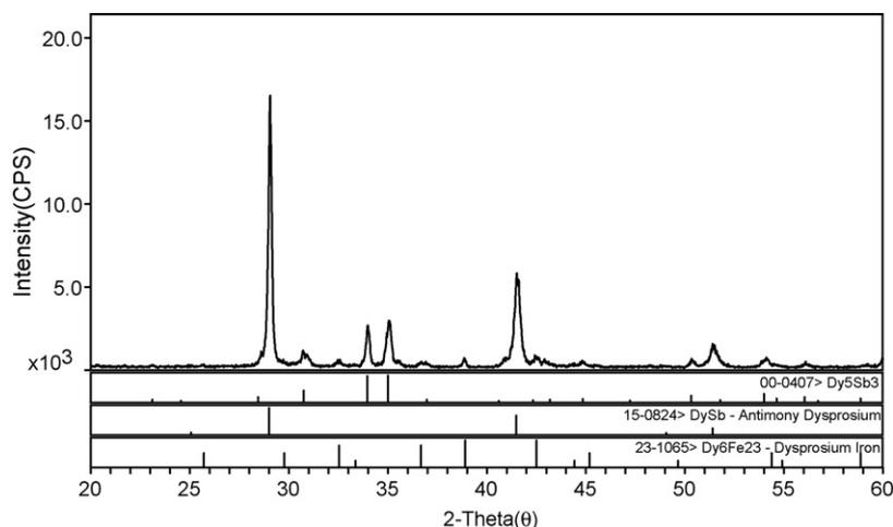
Fig. 2. XRD of the sample with composition  $\text{Fe}_{35}\text{Dy}_{41}\text{Sb}_{24}$ :  $\text{Dy}_5\text{Sb}_3 + \text{DySb} + \text{Fe}_{23}\text{Dy}_6$ .
