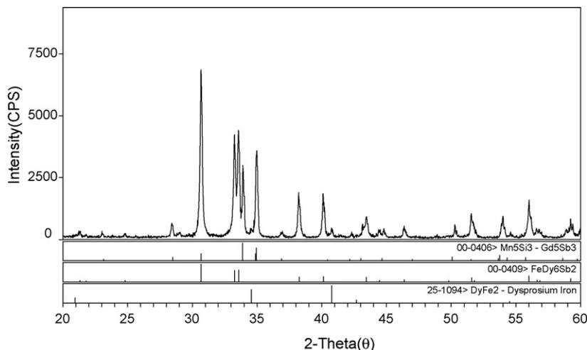
Fig. 4. XRD of sample with composition  $\text{Fe}_{11}\text{Dy}_{65}\text{Sb}_{24}$ :  $\text{Dy}_5\text{Sb}_3 + \text{Fe}_2\text{Dy} + \text{FeDy}_6\text{Sb}_2$ .
