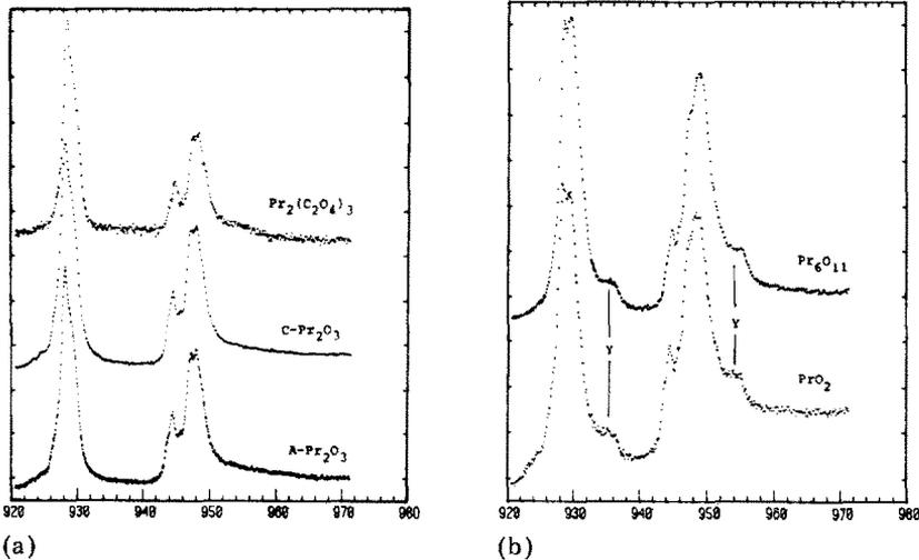
Fig. 2. (a)  $M_{IV-V}$  yield spectra of trivalent Pr compounds. (b)  $M_{IV-V}$  yield spectra of  $\text{Pr}_6\text{O}_{11}$  and  $\text{PrO}_2$ .
