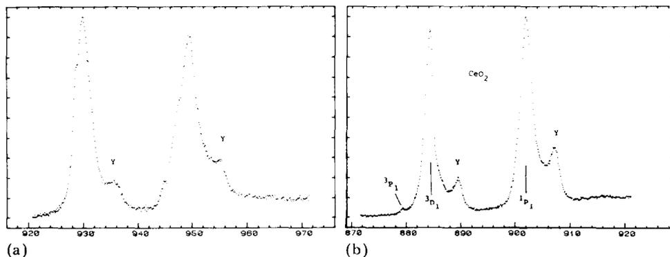
Fig. 3. (a)  $M_{IV-V}$  spectrum of tetravalent Pr obtained by subtraction procedure as described in the text. (b)  $M_{IV-V}$  yield spectrum of  $CeO_2$ .
