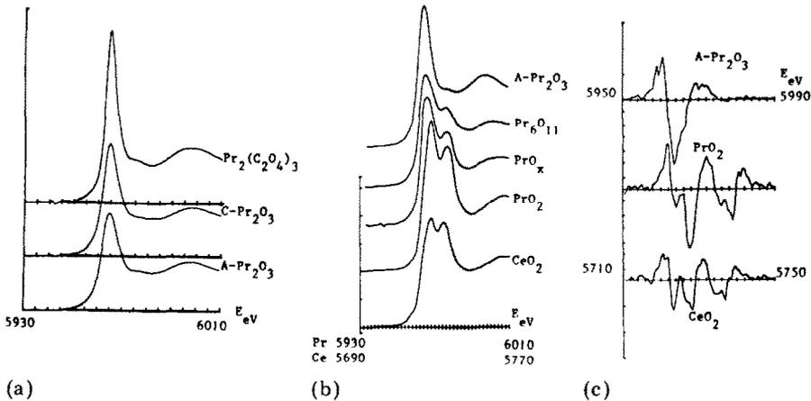
Fig. 1. (a)  $L_{III}$  absorption edges of trivalent Pr compounds. (b)  $L_{III}$  absorption edges of fluorite-structure-based Pr oxides. For comparison, the  $L_{III}$  edge of  $\text{CeO}_2$  is also included. Two different scales for Pr (5930 - 6010 eV) and for Ce (5690 - 5770 eV) are given. (c) Second derivative  $L_{III}$  spectra of C- $\text{Pr}_2\text{O}_3$ ,  $\text{PrO}_2$  and  $\text{CeO}_2$  with different energy scales for Pr and Ce.
