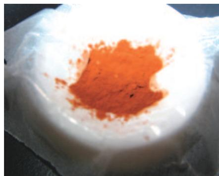
Fig. 1. Photograph of fullerodendron/CaCO<sub>3</sub> composite.
