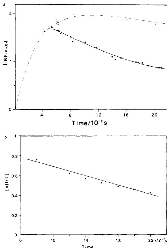
**Figure 5.** (a) Comparison of the decay of  $\text{NF(a)}$  in a coated (O) and uncoated (●) reactor for  $[\text{NF(a)}] \approx 5 \times 10^{11}$  molecules  $\text{cm}^{-3}$  and 3 Torr pressure. (b) A logarithmic comparison of the  $[\text{NF(a)}]$  in the coated and uncoated flow reactor versus reaction time. See text for details.
