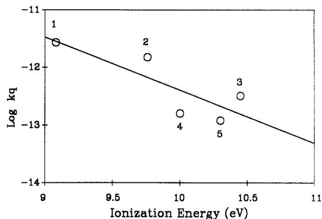
**Figure 12.** Correlations plot between the ionization energies of olefins and their quenching rate constants for  $NF(a)$ : 1,  $C_4H_6$ ; 2,  $C_3H_6$ ; 3,  $C_2H_4$ ; 4,  $CH_2CHCl$ ; 5,  $CH_2CF_2$ .
