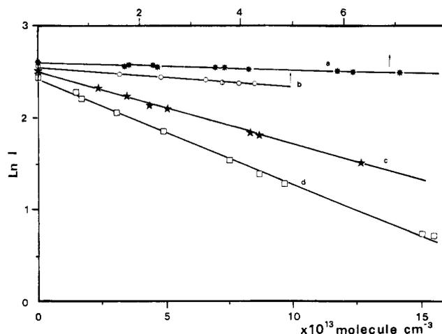
Figure 8. Pseudo-first-order NF(a) quenching plots for H<sub>2</sub>O (\*), D<sub>2</sub>O (O), CH<sub>3</sub>OH (★), and CH<sub>3</sub>OD (□) with reaction times of 106, 35, 79, and 83 ms, respectively. The units of the upper and lower concentration scales are the same.
