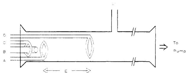
**Figure 1.** Schematic drawing of the 6.4 cm diameter flow reactor. A, B, C and D are the inlets for  $\text{HN}_3$ , F atoms, Ar buffer gas, and reagent, respectively; E denotes the prereactor section and F indicates pressure measurement. The distance between the  $\text{HN}_3$  inlet and the reagent inlet was 20 cm. The entire reactor was coated with halocarbon wax.
