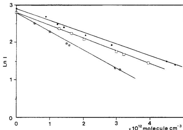
**Figure 9.** Pseudo-first-order NF(a) quenching plots versus concentration for three amines: ( $\square$ ,  $\text{CH}_3\text{NH}_2$ )  $\Delta t = 21$  ms; ( $*$ ,  $(\text{CH}_3)_2\text{NH}$ )  $\Delta t = 19$  ms; ( $\star$ ,  $\text{N}(\text{CH}_3)_3$ )  $\Delta t = 21$  ms.
