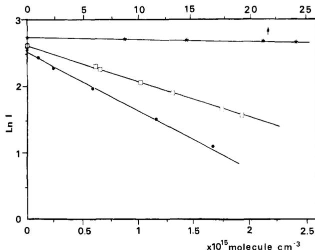
Figure 6. Representative pseudo-first-order NF(a) quenching plots for some diatomic reagents. The reaction times were 0.253, 0.175, and 0.153 s for N<sub>2</sub> (\*), CO (□), and O<sub>2</sub> (●), respectively. The  $[F]_0$  and  $[HN_3]_0$  were (26 and 3.8, 17 and 2.6, 20 and 7)  $\times 10^{11}$  molecules  $cm^{-3}$  for the N<sub>2</sub>, CO, and O<sub>2</sub> experiments, respectively.
