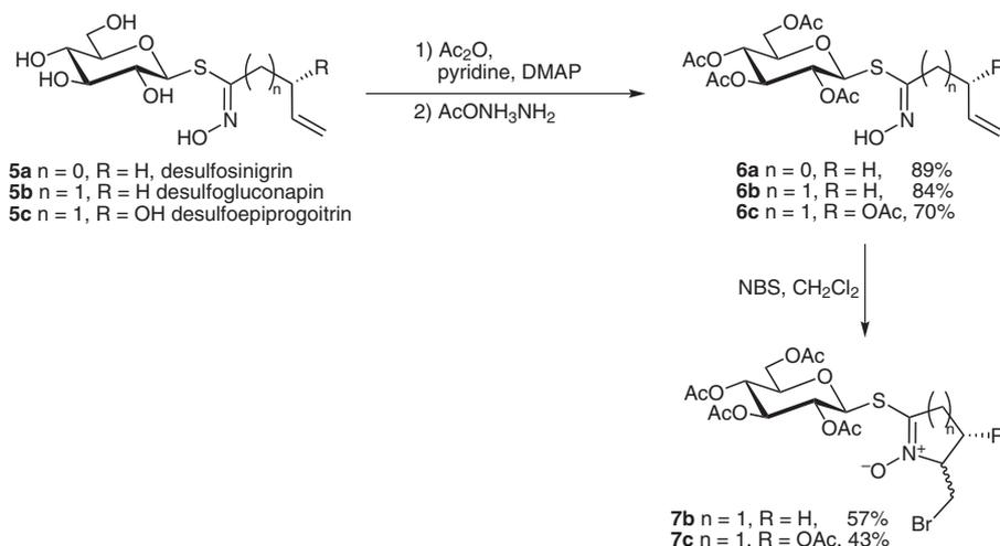
**Scheme 3** TIO derived from desulfoglucosinolates through halocyclization
