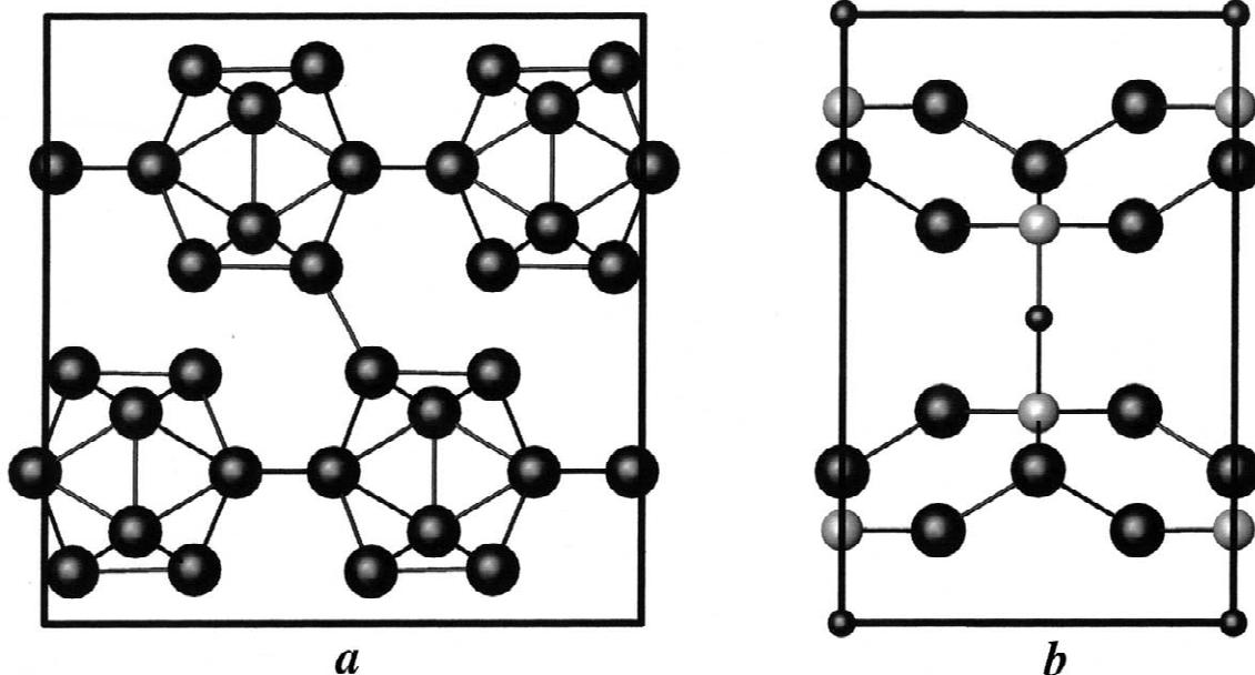
Fig. 4. Arrangement of the  $\text{B}_{12}$  icosahedra (a) and interconnection between hexagonal layers (b) in the  $\text{Al}_{0.185}\text{B}_6\text{CN}_{0.256}$  structure.
