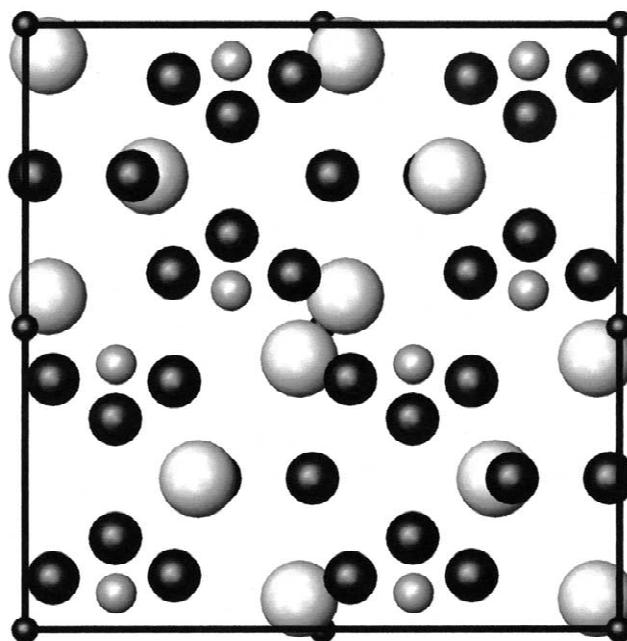
Fig. 3. Projection of the  $\text{Al}_{0.185}\text{B}_6\text{CN}_{0.256}$  structure onto the YZ plane (white large circles mean Al atoms, black middle size circles are used for boron atoms, grey small circles for carbon atoms and black small ones for nitrogen atoms).
