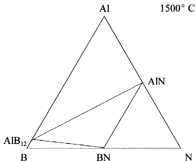
Fig. 2. Isothermal section of the Al–B–N system at 1500 °C.
