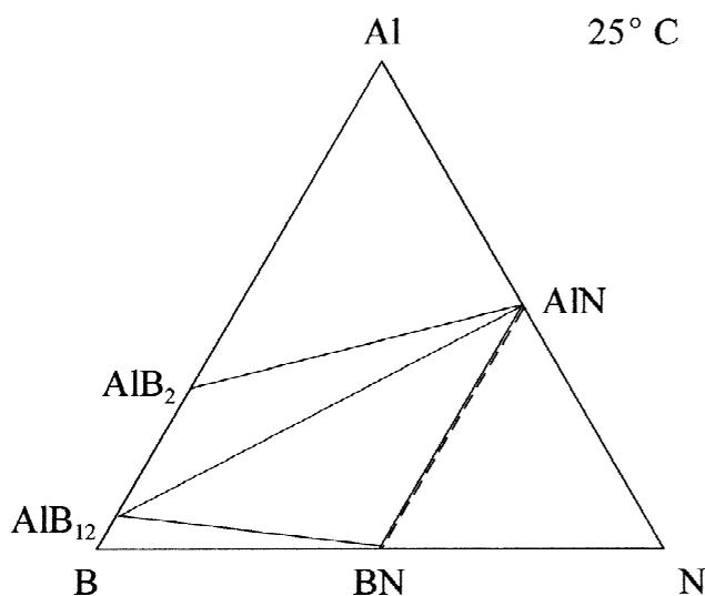
Fig. 1. Isothermal section of the Al–B–N system at 25 °C.
