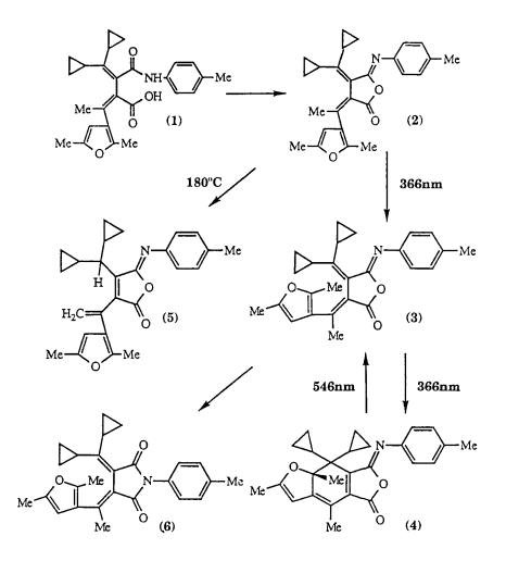
On irradiation with 366nm light the (Z)-isofulgimide (2) isomerized into the (E)-isofulgimide (3) which underwent a photochemical cyclization to give the coloured 7,7a-dihydrobenzofuran (4) ( $\lambda$  max 502nm in toluene). When this was irradiated with visible light the (E)isofulgimide (3) was regenerated. When the (Z)-isofulgimide (2) was heated at 180°C (CDCl<sub>3</sub> sealed tube) it underwent a [1,5]-hydrogen shift to give the isomaleimide (5).
