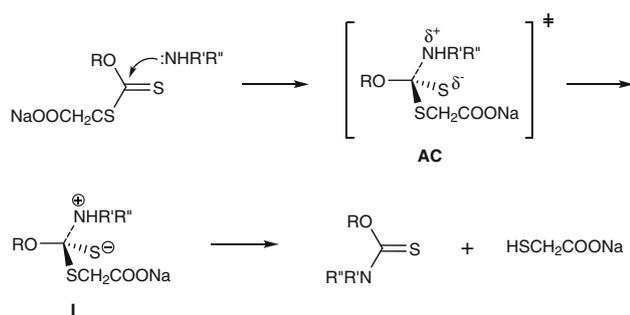
**Fig. 1** The most probable reaction pathway (AC activated complex, I intermediate) [15, 16]
