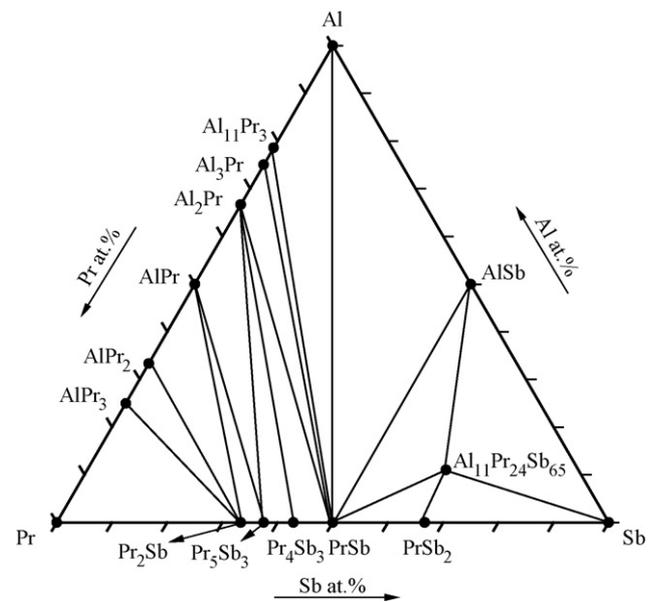
Fig. 4. The isothermal section of the Al–Pr–Sb system at 773 K.
