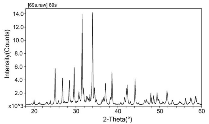
Fig. 3. X-ray powder diffraction patterns of  $\sim\text{Al}_{11}\text{Pr}_{24}\text{Sb}_{65}$ .
