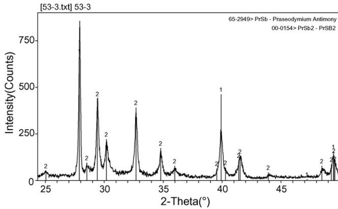
Fig. 1. Sample (40 at.% Pr, 60 at.% Sb) consists of PrSb (No. 1) + PrSb<sub>2</sub> (No. 2) two phases.
