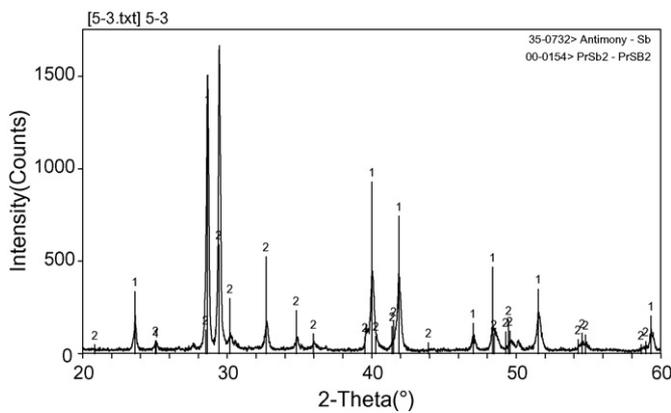
Fig. 2. Sample (20 at.% Pr, 80 at.% Sb) consists of Sb (No. 1) + PrSb<sub>2</sub> (No. 2) two phases.
