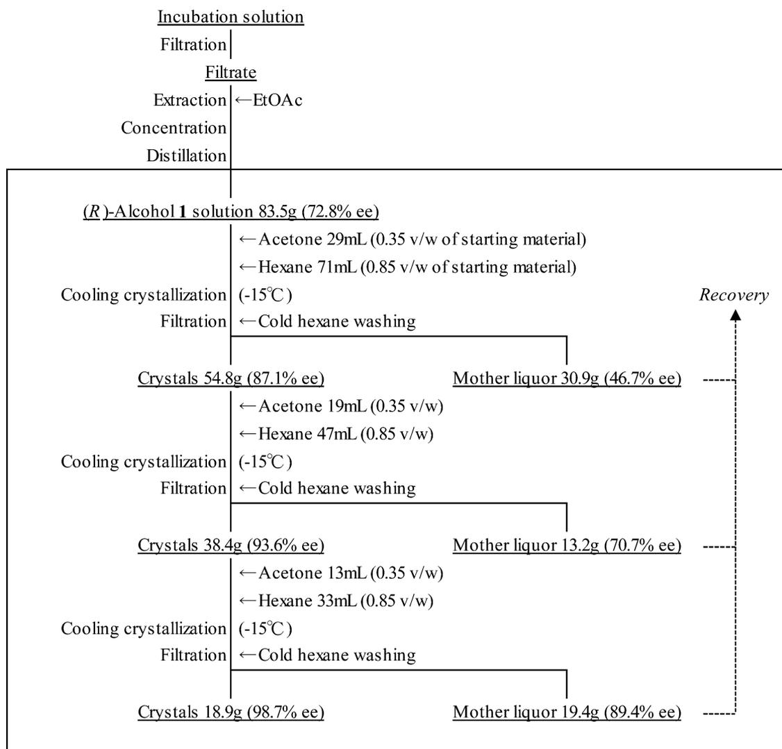
**Figure 1.** Crystallization flow for obtaining (R)-alcohol 1 with high optical purity.
