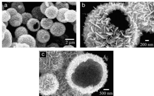
Fig. 4. Scanning electron microscopy images of the WO<sub>3</sub> hollow spheres (a, b) before, and (c) after sonication.
