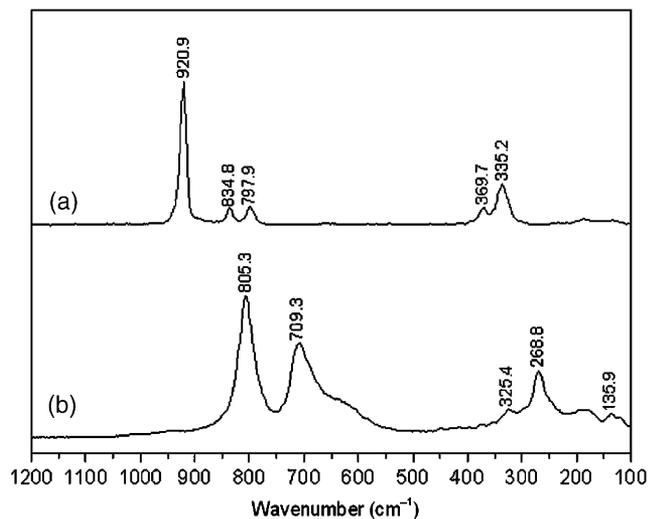
Fig. 5. Raman spectra of (a) SrWO<sub>4</sub>, and (b) WO<sub>3</sub> hollow spheres.
