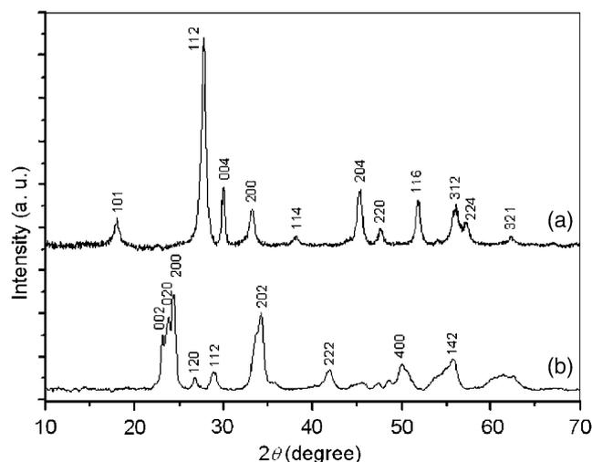
Fig. 1. X-ray diffraction patterns of the as-prepared (a)  $\text{SrWO}_4$ , and (b)  $\text{WO}_3$  samples.
