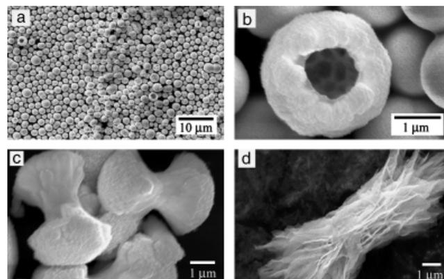
Fig. 3. Scanning electron microscopy images of (a) the typical as-prepared  $\text{SrWO}_4$  product, (b) magnified image of a hollow sphere; products obtained from controlled experiments, (c) when polymethacrylic acid (PMAA) was not present, and (d) when the pH value was 4 in the presence of PMAA.
