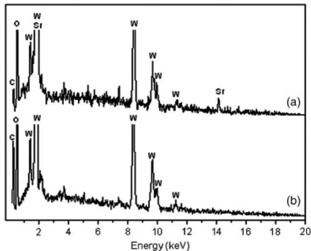
Fig. 2. Energy-dispersive X-ray spectrometry spectra of the as-prepared (a)  $\text{SrWO}_4$ , and (b)  $\text{WO}_3$ .
