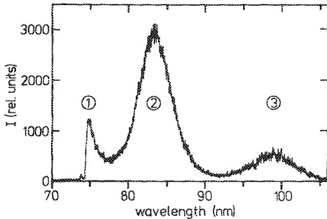
FIG. 2. Time-integrated emission spectrum of Ne at a pressure of 38.5 kPa. The first (1), second (2), and third (3) excimer continua were observed. The spectrum is corrected for the detection efficiency of the channeltron detector, but is not for the spectral response function of the monochromator.
