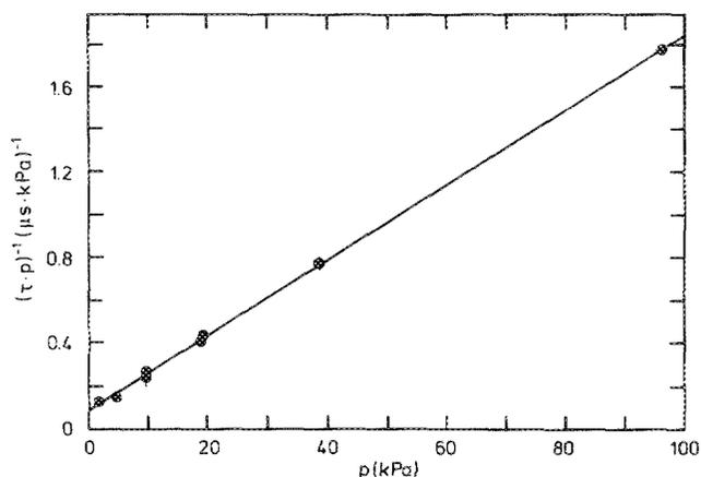
FIG. 4. Inverse of  $(\tau(p) \times p)$  is plotted vs the pressure  $p$  of the neon target in the pressure range between 1.8 and 96.1 kPa at an emission wavelength of 99 nm. Where no error bar is shown, the experimental error was smaller than the data point indicated. The straight line is a least-squares fit to the data.
