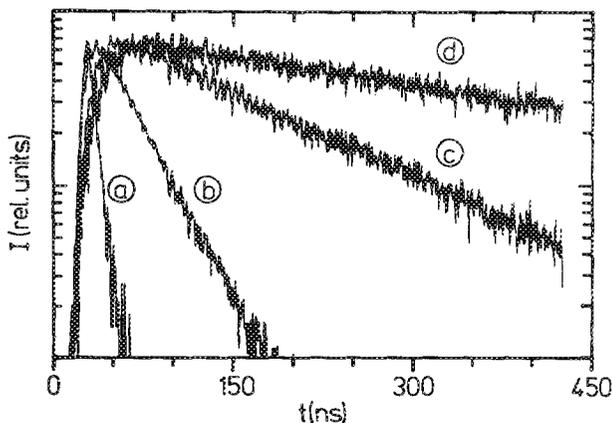
FIG. 3. Time spectra of the third excimer continuum in Ne at a wavelength of 99 nm. The spectra were taken with the setup shown in Fig. 1 at target gas pressures of (a) 96.1 kPa, (b) 38.5 kPa, (c) 18.6 kPa, and (d) 9.6 kPa.
